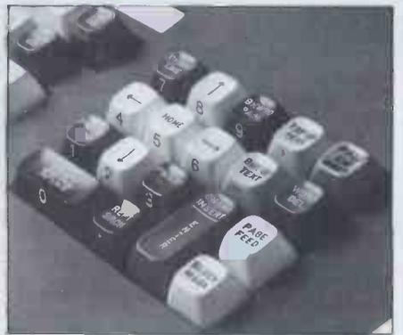
The special function keys, which replace the SuperBrain's numeric pad.
