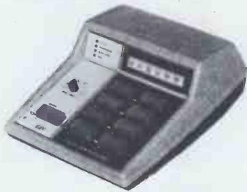
This unit provides simple, reliable programming of up to 8 EPROMS simultaneously it has been designed for ease of operator use — a single 'program' key starts the self check — blank check — program — verify sequence.
