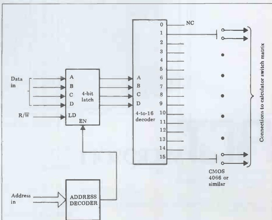
Fig 2 Block diagram of interface system
