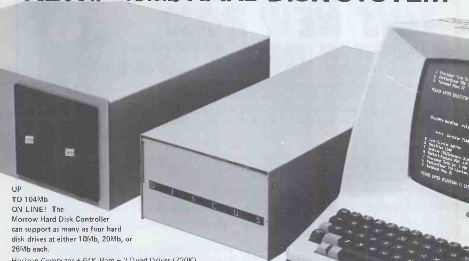
UP TO 104Mb ON LINE! The Morrow Hard Disk Controller can support as many as four hard disk drives at either 10Mb, 20Mb, or 26Mb each.
