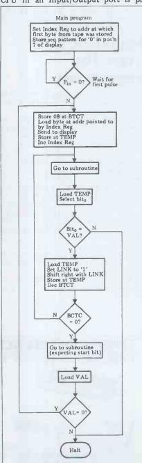
Program 3 Comparing a program loaded from tape into RAM with the tape program. The subroutine and hardware are the same as in Program 2
