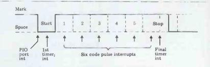
Fig 1 Baudot code signal timing diagram, showing interrupt times. Most commonly-used pulse length is 20 ms for start and code pulses, 30 ms for stop pulse (50 baud)
