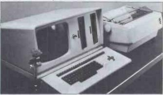
This very neat machine is called the Caltext, a British-made word processor from Computer Ancillaries Ltd, which costs an amazing £3995, complete with 64k RAM, twin disks and a daisywheel printer. But the Caltext isn't quite what it seems, for it runs Wordstar under CP/M, which means you've only got to slot in a different disk and you can run all sorts of other CP/M-based software. More on Egham 36455.
