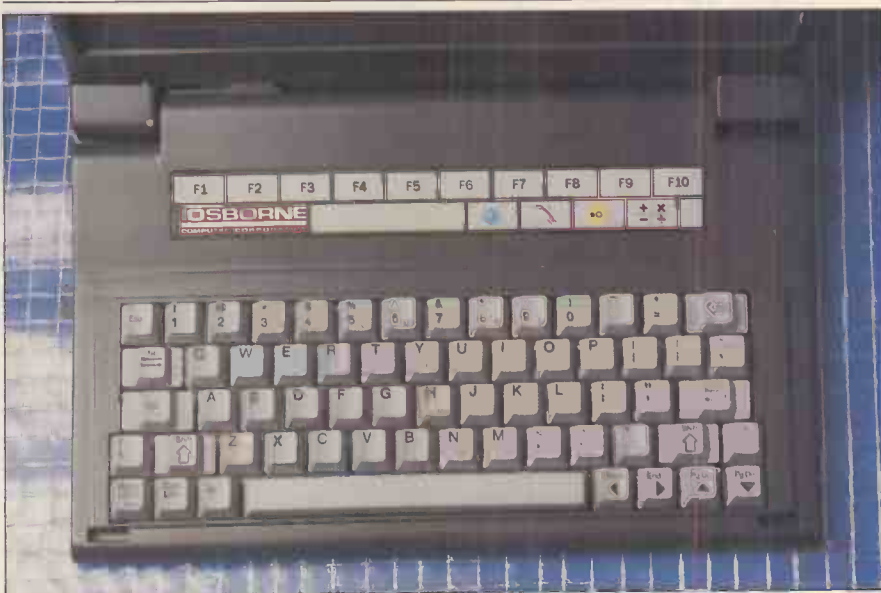
63 proper typewriter keys; note the four brightly coloured icon-style function keys
