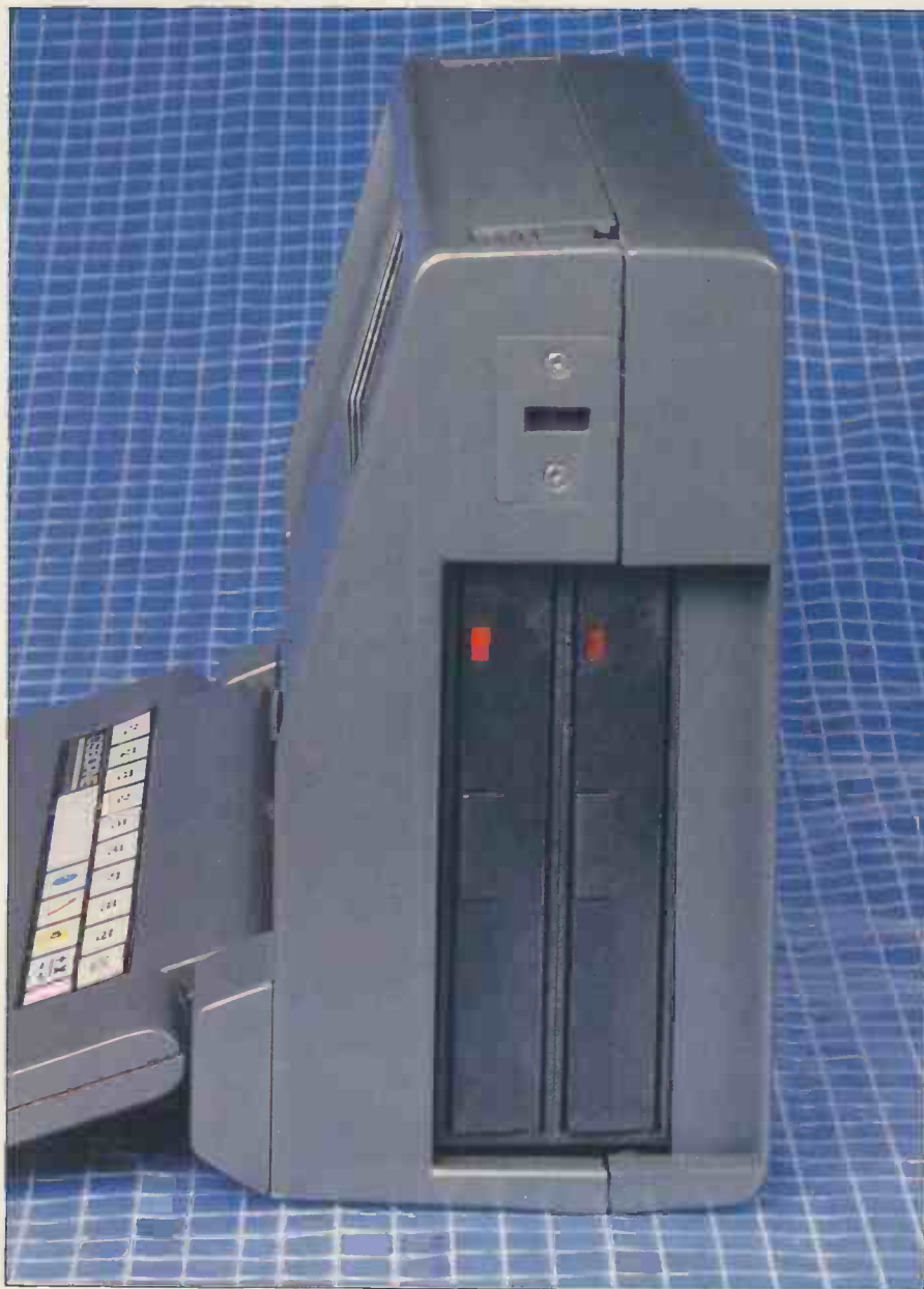
New design 5¼in disk drives; the second disk drive is an optional extra
