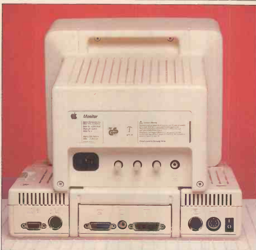
The back panel is crowded and houses a dual-purpose handle
