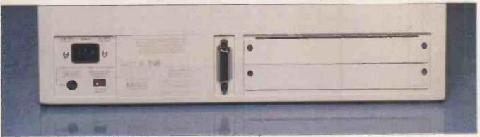
The back of the machine supports just one true interface — the standard IEEE-488 HP-IB bus
