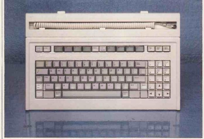
The low-profile detachable qwerty keyboard has 90 keys, a good feel and a tilt mechanism
