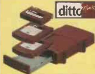
The Iomega Ditto drive allows you to customise your capacity because its unique cartridge caddy takes a choice of 3.5Gb, 5Gb, 7Gb and 10Gb tape cartridges, as well as reading smaller TR-3 and 2Gb cartridges.
