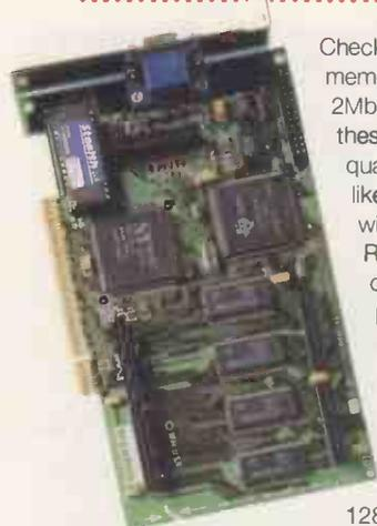
Check the amount of memory on the card. 2Mb is standard these days. Better-quality cards are likely to be fitted with VRAM (Video RAM). Also, check out the performance capability of the card. Video cards come as 16-bit, 32-bit, 64-bit and even 128-bit: a large
