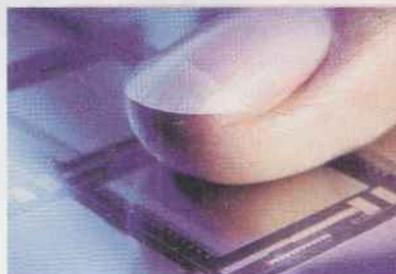
Siemens (01344 396 396) reckons it has its finger on the pulse of security with this sensor which packs a fingerprint digitiser onto a single chip to identify users.
