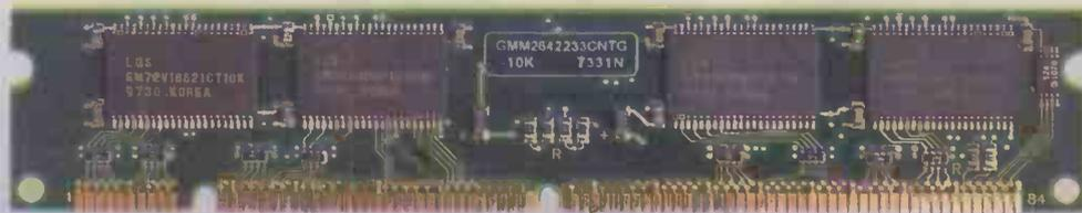
168 pin Un-Buffered DIMM 3.3v (SDRAM)
