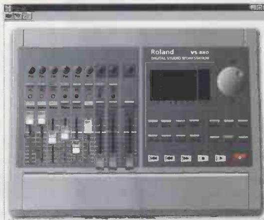
**Fig 1** Cakewalk's StudioWare provides on-screen panels for synths and digital audio workstations like the Roland VS-880
