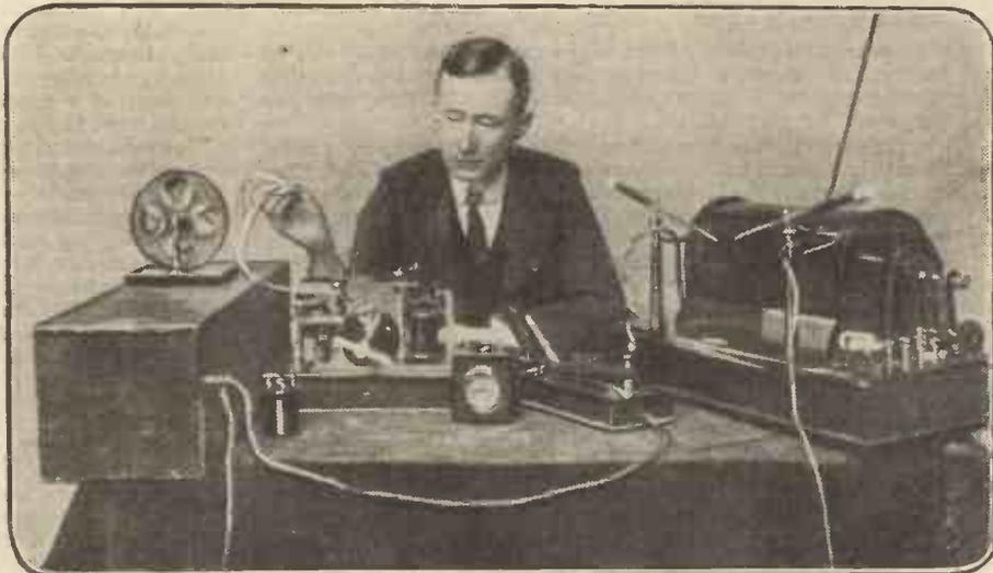
Our photograph shows Mr. Marconi with one of his earliest transmitting and receiving sets. Note the 10' spark coil, and the old-fashioned tape recorder used in conjunction with the coherer detector.
