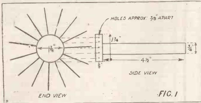
spokes and is now ready for winding the first coil (Fig. 1).
