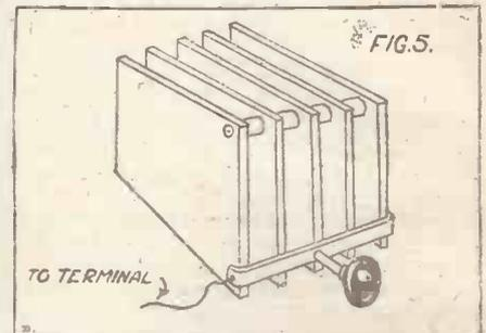
square; 6 pieces of paraffin-waxed paper,  $1\frac{1}{2}$  in. square; and two pieces of  $\frac{1}{8}$ -in. ebonite, 2 by  $1\frac{1}{2}$  in. Four  $\frac{1}{2}$ -in. brass screws will do for securing the parts together.
