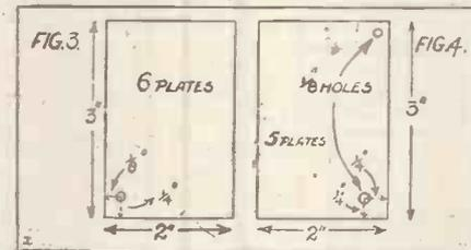
through one corner, the centre of which should be  $\frac{1}{8}$  in. from one edge and  $\frac{1}{4}$  in. from the other (Fig. 3). Now clamp the remaining five plates, and drill a  $\frac{1}{8}$ -in. hole through each corner on the 3-in. side, the centre to be  $\frac{1}{8}$  in. from each edge.
