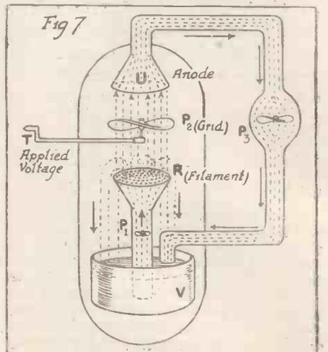
main propeller H revolving at the same speed. The distance between U and R weakens the suction effect on water emerging from the rose R; but the propeller  $P_2$ , being quite close to R, has a very big effect on the quantity of water sucked up into the funnel U.
