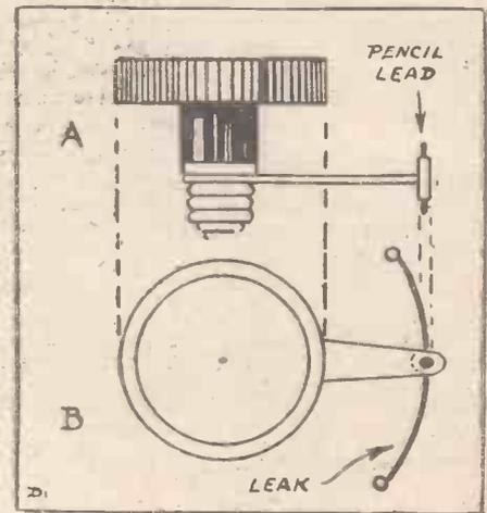
The pencil lead should make just sufficient contact with the leak to ensure a good connection, and should not be pressed tightly on to the leak, for obvious reasons.
