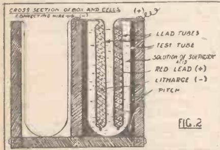
then filled with red lead and the other with litharge, the open ends being squeezed for  $\frac{1}{8}$  in. to close them up. The positive tube will be the one filled with red lead (oxide of lead); 16 tubes with red lead and 16 with litharge will be required.
