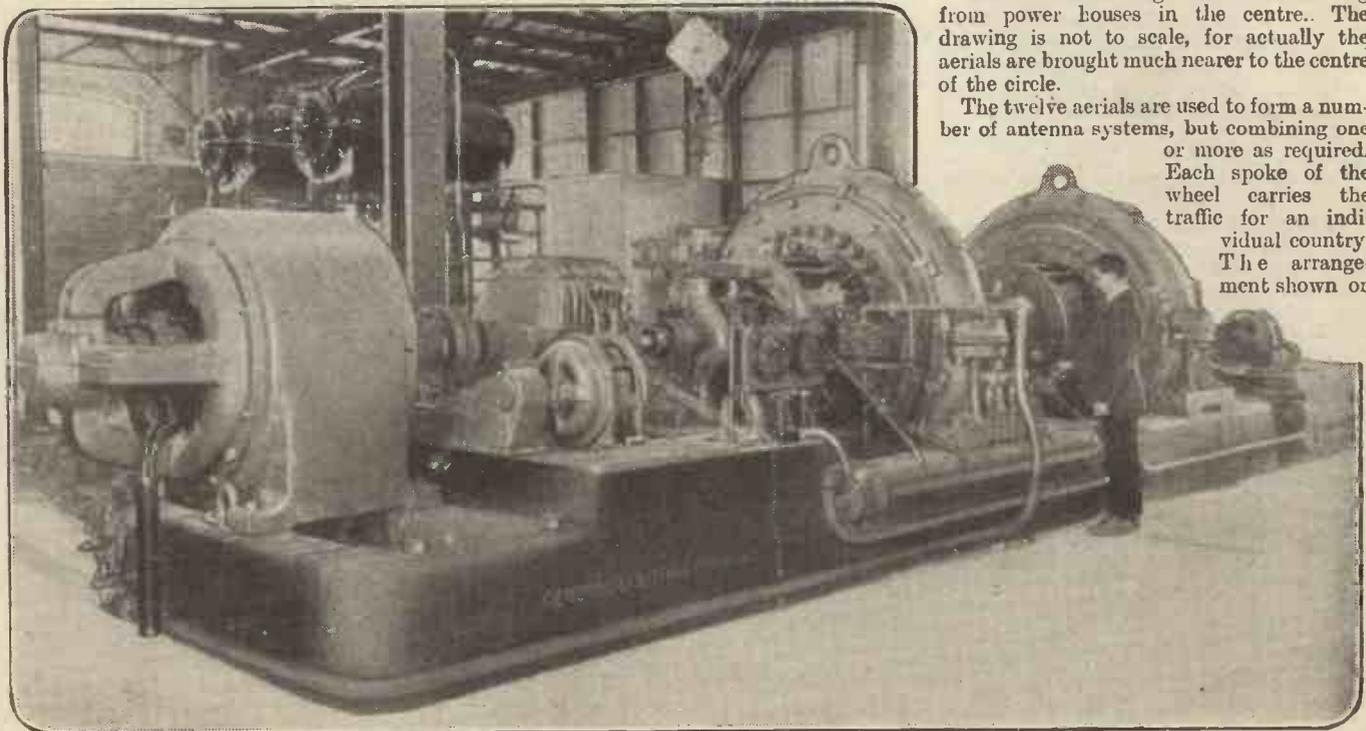
One of the huge Alexanderson alternators at Radio Central. Each alternator has an output of 200 k w.
