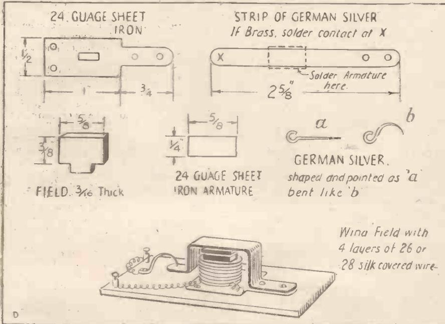
Making a Small Testing Buzzer.
