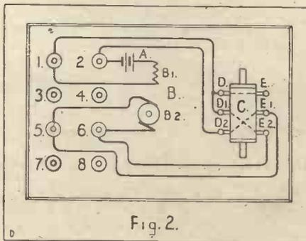
The polarity of the current traversing the field magnet winding B1 would, however, remain unaltered, so that the armature with commutator B2 would revolve in a reverse direction to that previously described.
