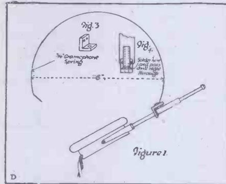
in more than uncomfortable and ill-fitting phones. To fit snugly but firmly to the ears each phone must have some sort of "universal motion" This is simply and effectively provided by what is known as the "stirrup and gymbal."
