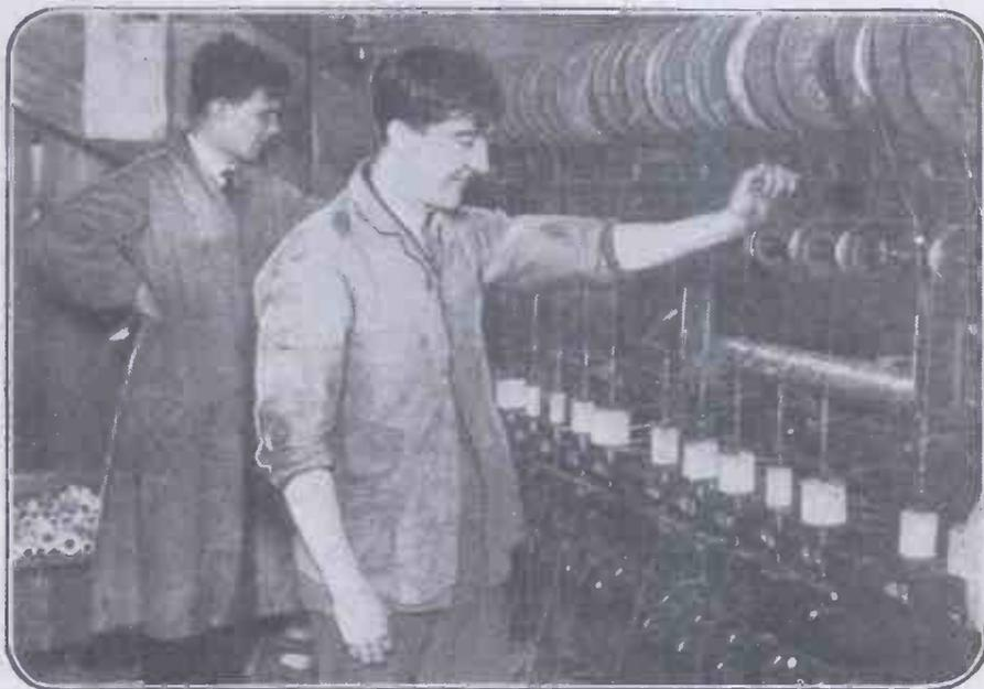
Covering wire with silk and cotton insulating material in a large wireless works at Acton.
