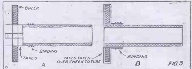
When this is done the core may be inserted in the bobbin, the first binding wire should not be removed to prevent the wires fanning out, but all the others should be removed as the core is inserted. When the core has been pushed through the bobbin, the first binding wire may be removed and the core adjusted to project equally either side.
