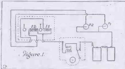
have purposely included several unnecessary markings which only serve to make a diagram more incomprehensible and difficult to follow. In the first place let us remove all superfluous markings and, using the conventional sign for the battery, we have quite a different and clearer view of the same circuit (see Fig. 2).
