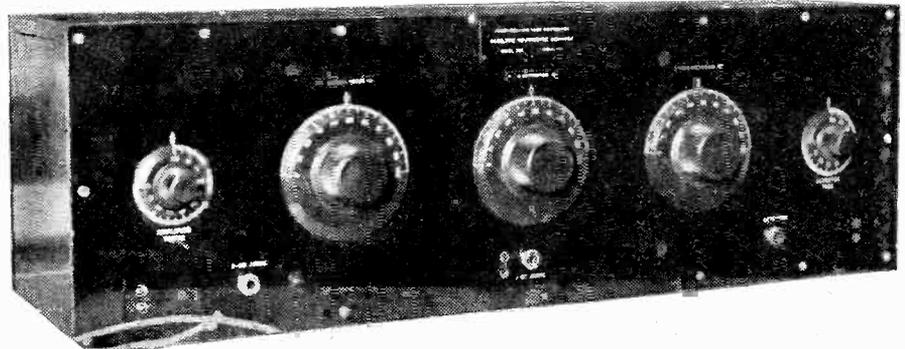
The external appearance of the Neurodyne Receiver. The dial on the extreme left controls all the amplifying valves, no potentiometer being used, while the next dial controls the aerial tuning adjustment. The third and fourth are "neurostages," and the last the detector valve control.
