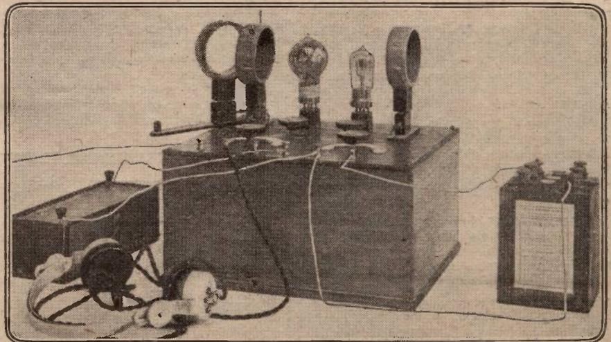
Fig. 6. The complete receiver ready for use.
