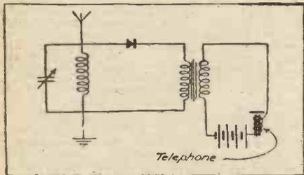
You say that coupled circuits give a step up of potential and stronger signals result. By actual measurement of 'phone current this is not the case. Moreover, no appreciable increase in selectivity occurs until the coils are so far separated that signal strength is badly reduced. If "tuning curves," such as the one reproduced in my article, be taken for close coupling and loose coupling of the coils, the shapes are absolutely similar.
