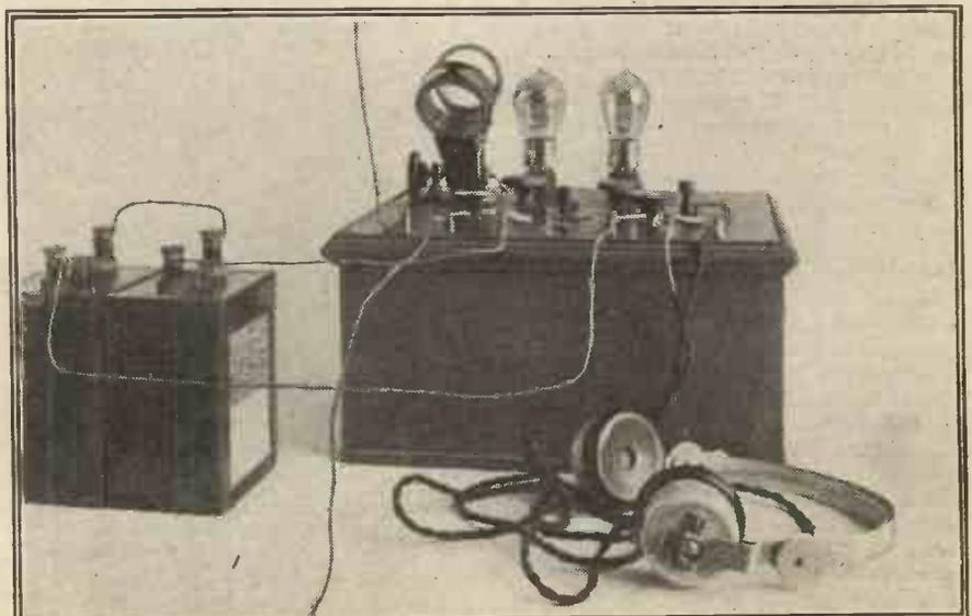
Fig. 2. The complete set ready for use. The absence of an H.T. battery is strikingly noticeable.
