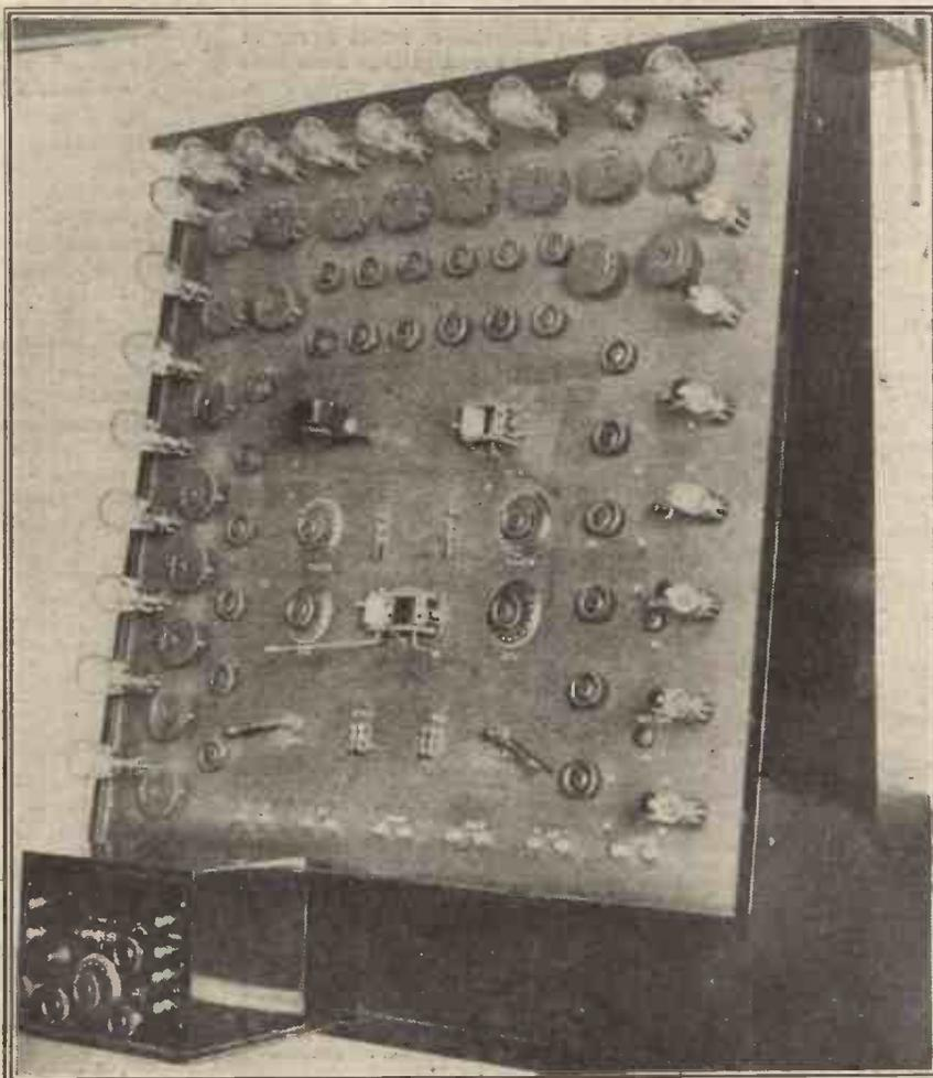
A special article dealing with the experiments made with the 24-Valve Set appears in this issue. Note the 2-Valve Unidyne Set in this photo, and compare the size of it with the 24-Valve Set!
