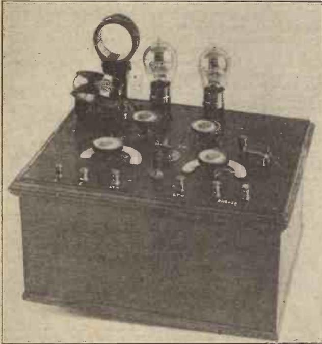
Fig. 3. Note the symmetrical lay-out of the panel and the accessibility of the tuning controls.
