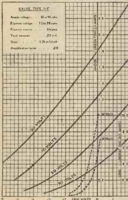
grid current is avoided. This permits the use of the valve without a grid bias, yet avoids the harmful distortion of speech that usually occurs under such conditions with valves possessing appreciable grid current.
