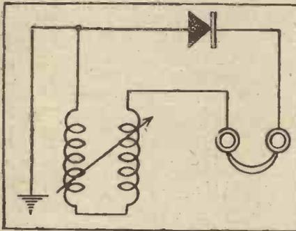
Good signals are heard 3 1/2 miles from 2 L O at the address below, using only the 'phone leads as an aerial. I have recently been making experiments with a view of constructing a set using aperiodic tuning, as different "earths" affect it in the same way as different aeriels would an ordinary receiver.
