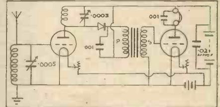
causes a current flow through the primary and crystal, so rectified impulses are passed on to the secondary of the L.F. transformer, which is connected to grid and filament of the last valve. This valve will thus act as a L.F. amplifier, with phones connected in its plate circuit.
