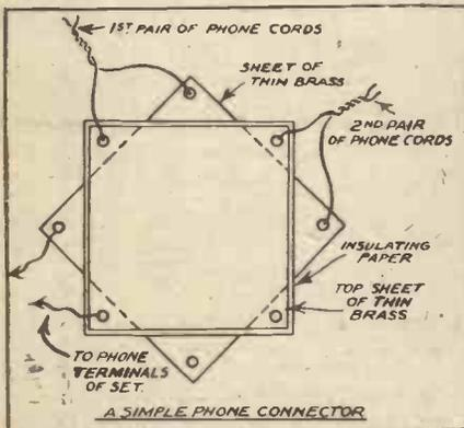
up to the set, but probably the one illustrated herewith is as simple as any. It consists of two small sheets of fairly thin gauge metal—brass sheet—cut with a number of projecting points.
