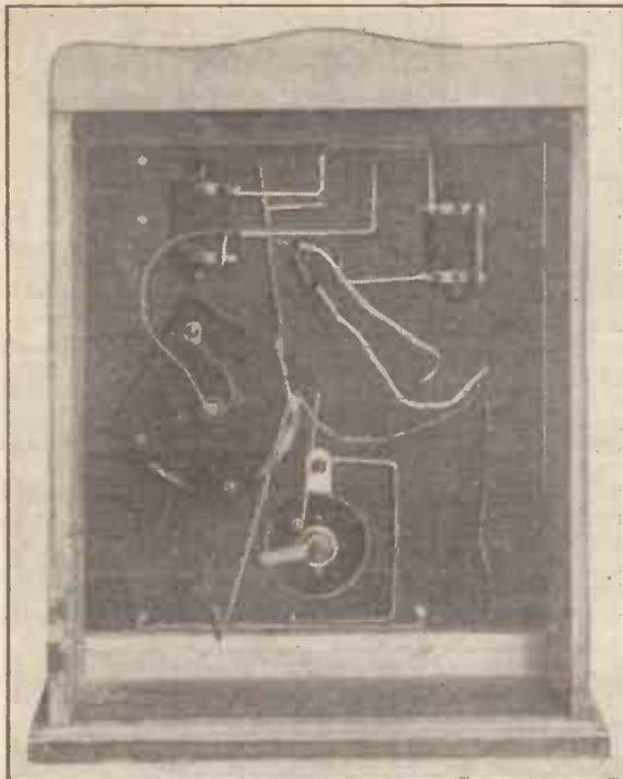
Fig. 5. The completed wiring of the set as seen through the glass back.
