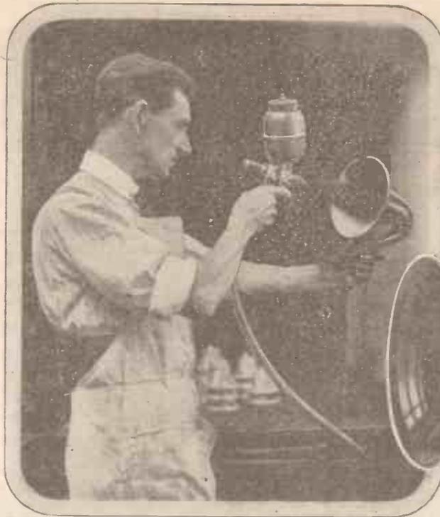
Illustration showing the horn of a Brown Loud Speaker being sprayed with enamel.
