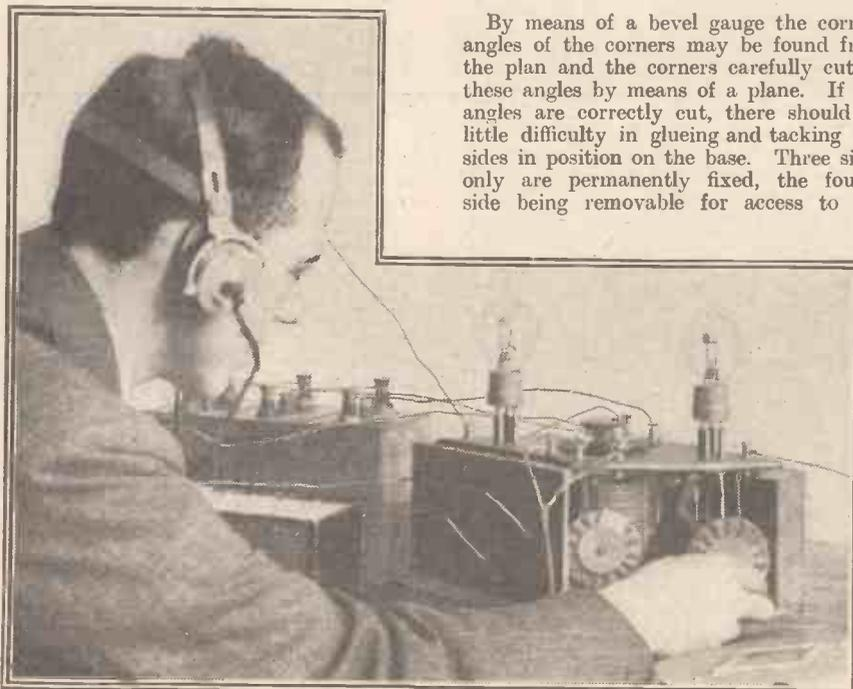
Fig. 6. The set in operation, showing adjustment being made to the reaction coil.
