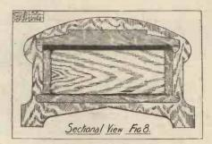
occupying but little space. The case can be made in oak, walnut, or mahogany, and nicely polished. An idea of its construction is given by Figs. 8 and 9. The ends are grooved into the sides; the bottom fits between them. The ebonite panel is fixed to the ends with small screws. Two small shaped strips of wood, fixed at the ends of the lid, prevent it from slipping off.
