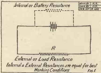
as follows: If a source of direct or alternating current having internal resistance is connected to a work or load circuit, then the maximum power is expended in the load (i.e. one gets the most useful working conditions) when the latter power is equal to the power consumed in the source itself.
