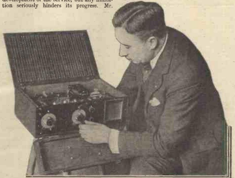
This completely self-contained American portable set is extraordinarily compact, as readers will agree when it is stated that an eight valve super-het circuit is employed.
