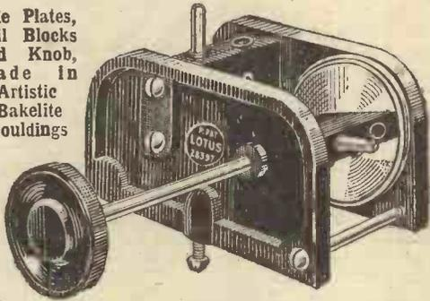
You have experienced that annoying and irritating fading away of volume after tuning your coils. This is due to the moving block falling. The Lotus Moving Block **CANNOT FALL**. The Vernier movement comprises three sets of enclosed precision machine-cut gears, and reduces the speed of the moving coil block by eight times.
