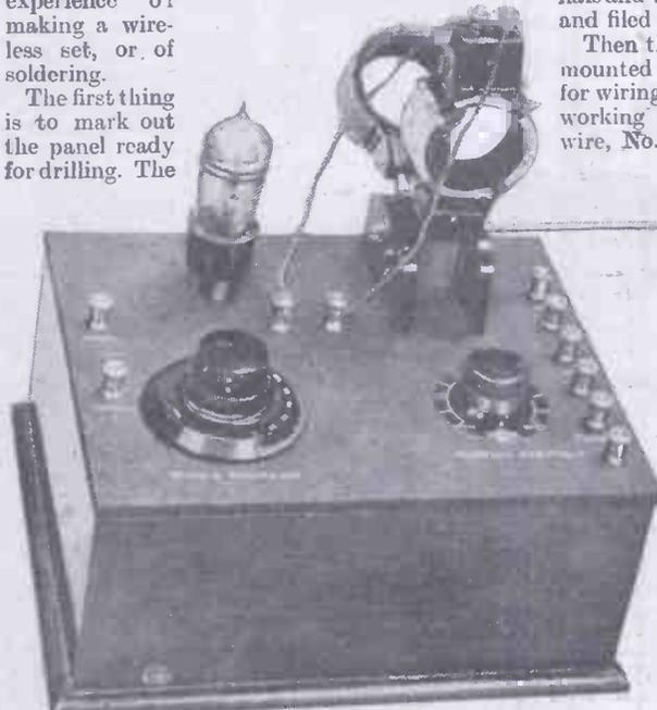
The flexible leads to the Ultrynic aerial coil are shown in this view of the complete receiver.
