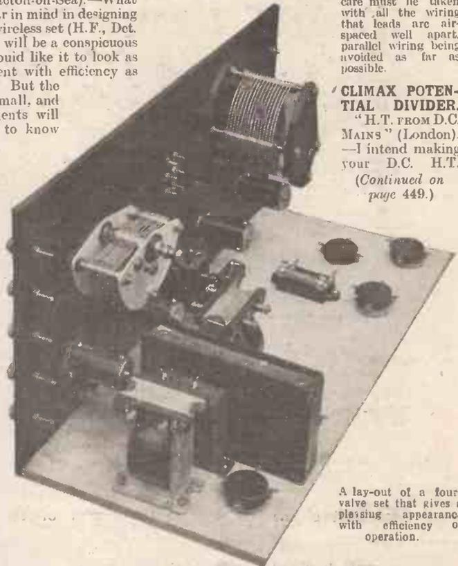
A lay-out of a four-valve set that gives a pleasing appearance with efficiency of operation.
