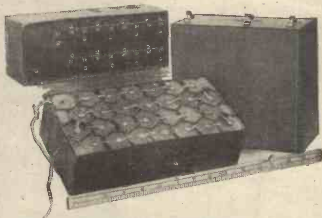
This illustration shows how the sizes of H.T. batteries differ. The smallest in size has the highest voltage.
