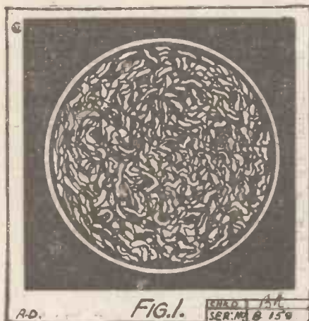
Greatly magnified bluish crust formed on accumulator terminals.
