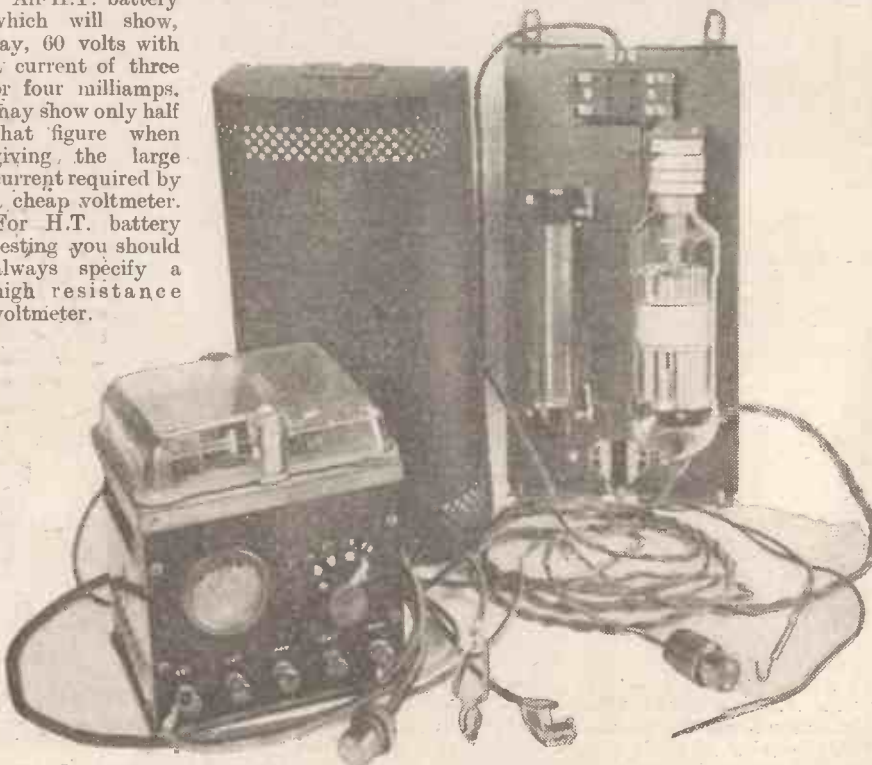
For those who wish to charge their H.T. accumulators at home, there are several commercial forms of charges, two of which are shown above.
