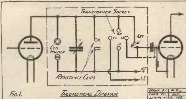
value of from 50,000 to 100,000 ohms, connected in the anode circuit, giving rise to voltage impulses on the grid of the second valve. The corresponding amplified variations in the plate current of this valve are handed on in a similar manner to the grid of the detector, or the next H.F. stage.
