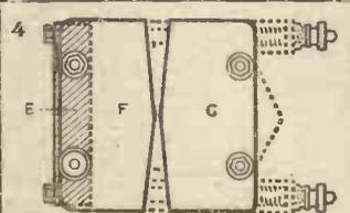
The fixed plates "F," carried on a high-grade ebonite insulating bar "E," and the moving plates "G" are now fitted, thus completing the instrument. In its finished form it occupies a space back-of-panel of only 3 1/2" x 2 1/4". The 4" Dial supplied is divided into 360 degrees.
