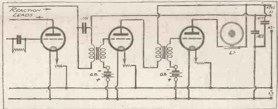
Fig. 1. A conventional transformer coupled arrangement. Compare this with the diagram below.
