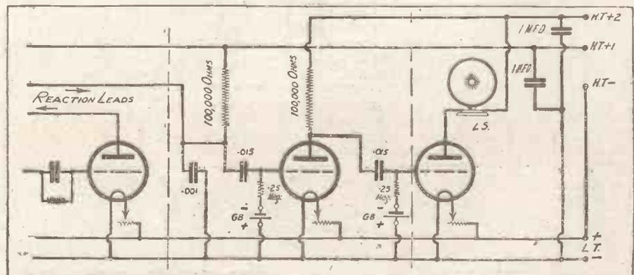
Fig. 2. A resistance amplifier unit. Note that the portions to the left and right of the dotted lines are the same as in the transformer coupled arrangement above.
