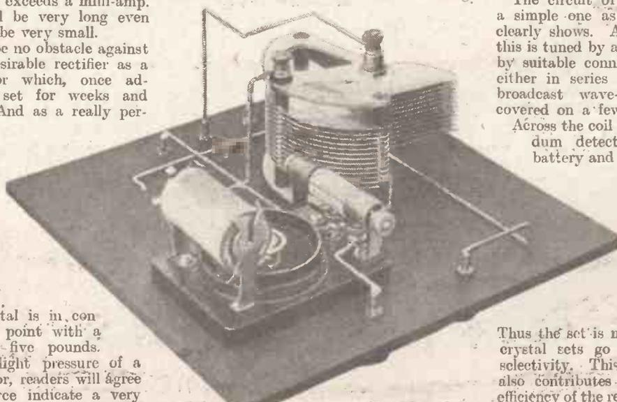
The carborundum detector unit can be clearly seen in this "under-panel" photograph.
