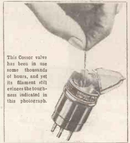
This Cossor valve has been in use some thousands of hours, and yet its filament still evinces the toughness indicated in this photograph.
