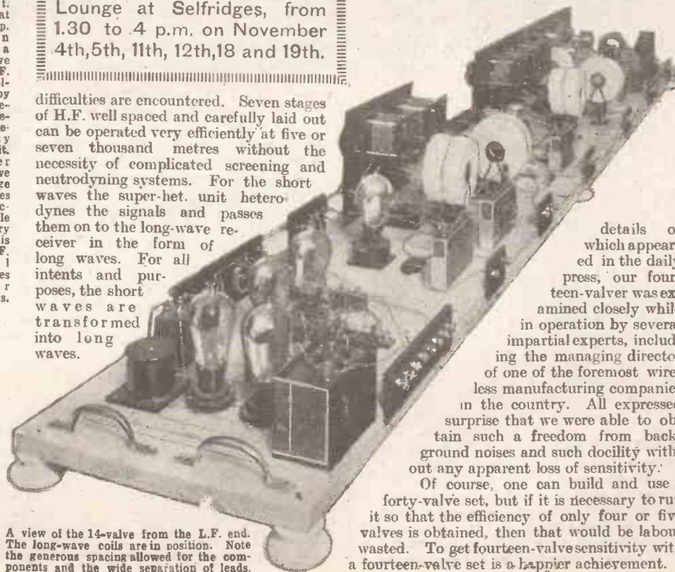
A view of the 14-valve from the L.F. end. The long-wave coils are in position. Note the generous spacing allowed for the components and the wide separation of leads.
