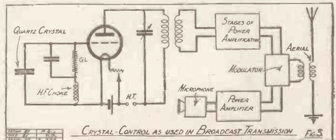
CRYSTAL-CONTROL AS USED IN BROADCAST TRANSMISSION Fig. 3.
