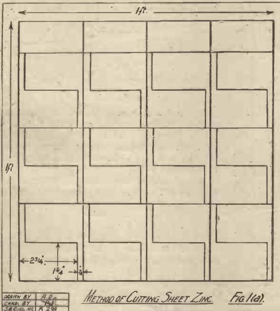
METHOD OF CUTTING SHEET ZINC. Fig. 1(a).
