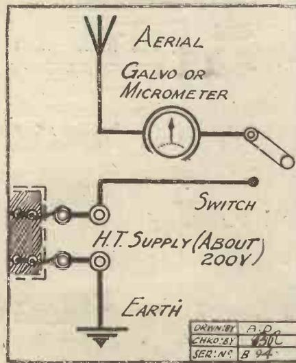
gradual loss in the aerial's insulation efficiency due to the sooting up of the insulators to be the prime cause of the mysterious trouble.
