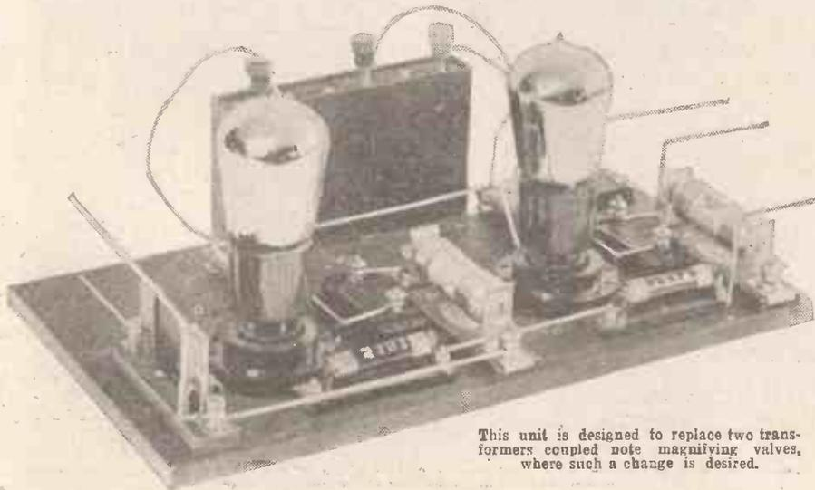
This unit is designed to replace two transformer-coupled note magnifying valves, where such a change is desired.
