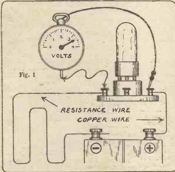
adjustments are necessary, for the valve will function efficiently at all times providing the accumulator is kept up to the mark. This means, of course, that we can use a very simple and compact form of fixed resistance or "resistor," in place of the usual variable resistance, or "rheostat," and the result is a great saving of space on the panel or baseboard of the set, and fewer control knobs. Moreover, a number of fixed resistors may be easily made up at home at a trifling cost.
