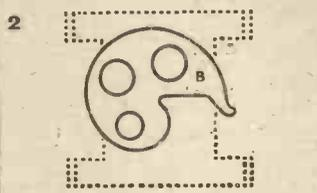
To this is added a Cam "B" according to the shape of which either S.L.F. or Square Law characteristics are obtained. The Cam drive gives a fine tuning ratio of approximately 5 to 1 over every part of the scale.
