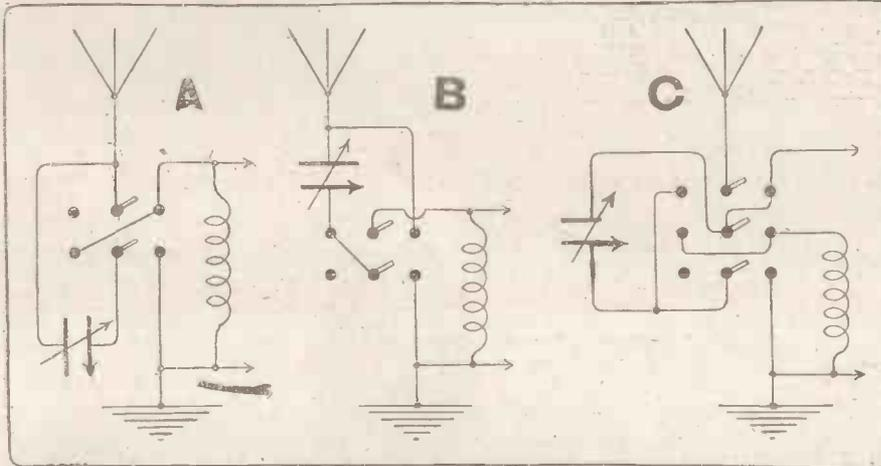
is thus placed in close proximity to the spindle, or otherwise moving vanes. For this reason they should always be connected to the "earthed end" of a circuit. In other words, the fixed vanes should be connected to the "aerial" or "grid end" of a circuit, not only in the case of direct or inductively coupled aerial circuits, but also in tuned anode and H.F. transformer couplings, the anode of the valve being considered as the "grid end" in the latter examples.
