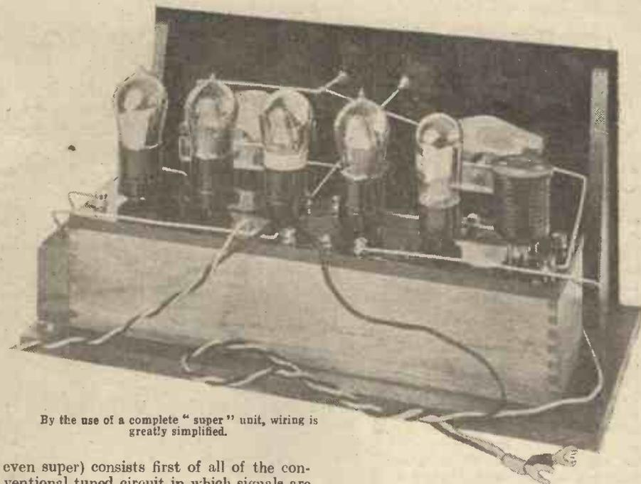
By the use of a complete "super" unit, wiring is greatly simplified.
