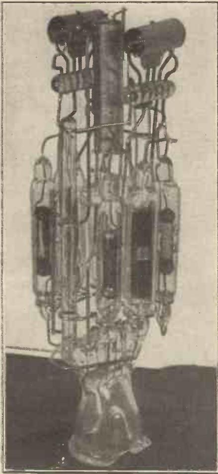
(Above). A "close-up" of the Loewe triple valve partially assembled.
