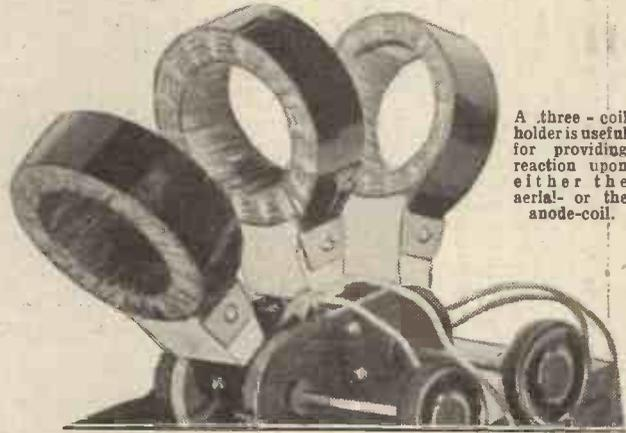
A three-coil holder is useful for providing reaction upon either the aerial- or the anode-coil.
