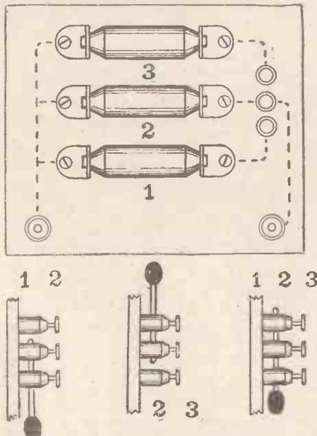
Fig. 4.—A very simple arrangement for three condensers.
