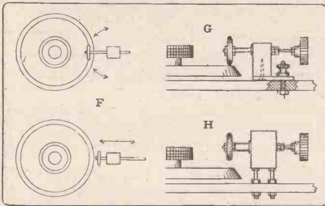
Fig. 4. A system of removable vernier controls.
