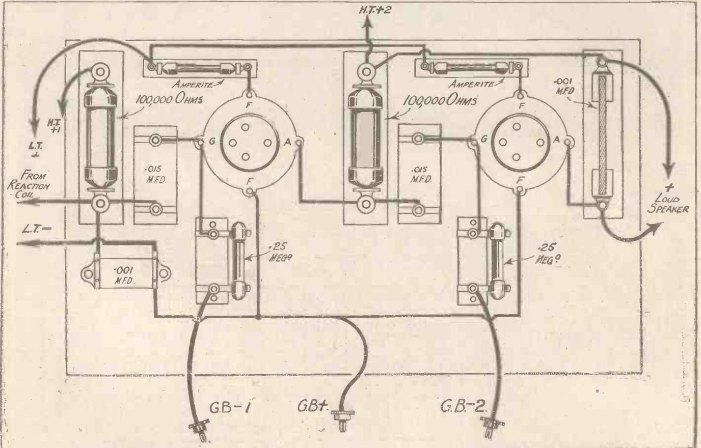
Fig. 4—This diagram shows both the wiring and the connections to the other parts of the apparatus. Mansbridge condensers should be obtained across the H.T. terminals, if not already fitted.
