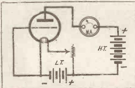
Fig. 1. Measuring plate current with a milliammeter.
