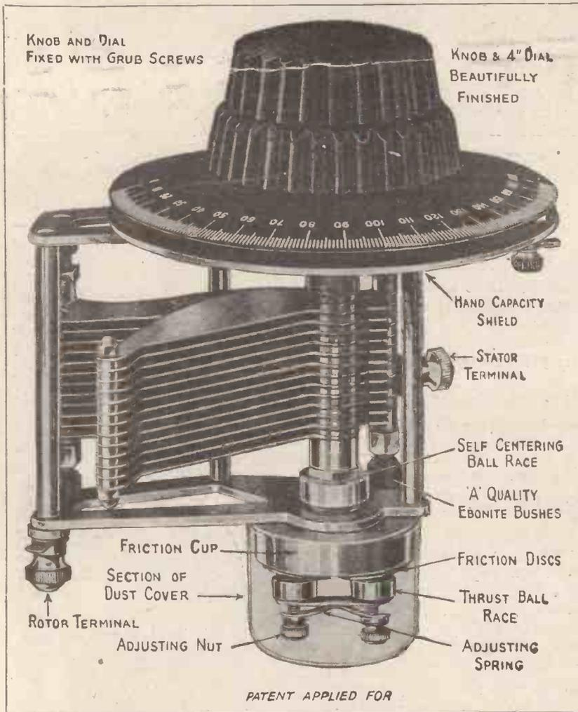
THE famous ORMOND SLOW MOTION FRICTION DRIVE (ratio 55-1) is incorporated and special ball bearings give liquid-like movement to every turn of the knob. It has an anti-capacity earthing shield which may be fitted, insulated from the condenser, and earthed by a separate connection. This world-famous ORMOND Component is easy to mount, having one and three holes for fixing, with both terminals and soldering tags for connections.
