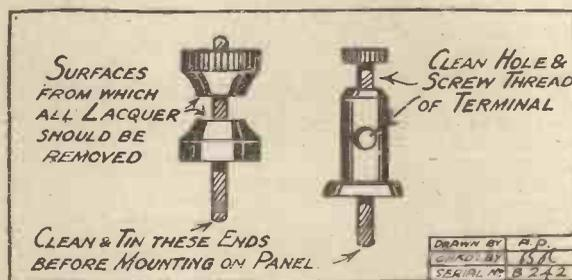
Screw down terminals, and terminals of the push-through type, require the lacquer
