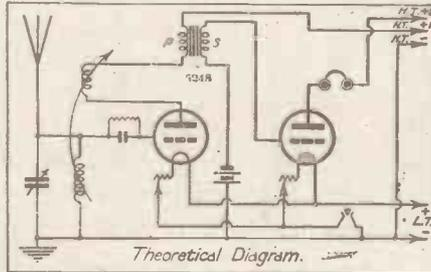
The diagram (reproduced herewith) shows the required arrangement. Grid bias and extra H.T. for the last valve have been incorporated. Although 'phones are shown in the plate circuit of the second valve, a loud speaker can be used here when the incoming signal is fairly strong. No 'phone or loud speaker condenser is shown, but of course this can be used if required.
