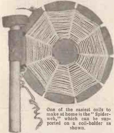
One of the easiest coils to make at home is the "Spider-web," which can be supported on a coil-holder as shown.
