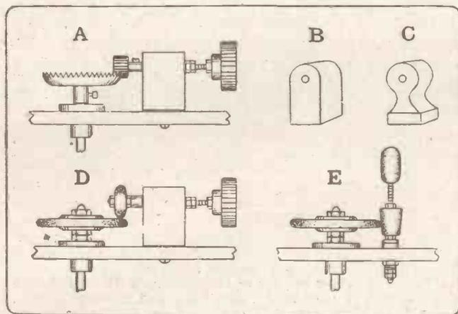
Fig. 1. Some simple methods of obtaining Vernier control.
