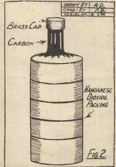
jar, and the zinc (negative) into the second jar, and so on to the end. The last jar is completed by placing a carbon only with soldering tag inside the zinc; this is the positive pole. Next fill the jars with ammonium chloride (sal ammoniac)—six ounces to one pint of water—and the battery is ready for use.
