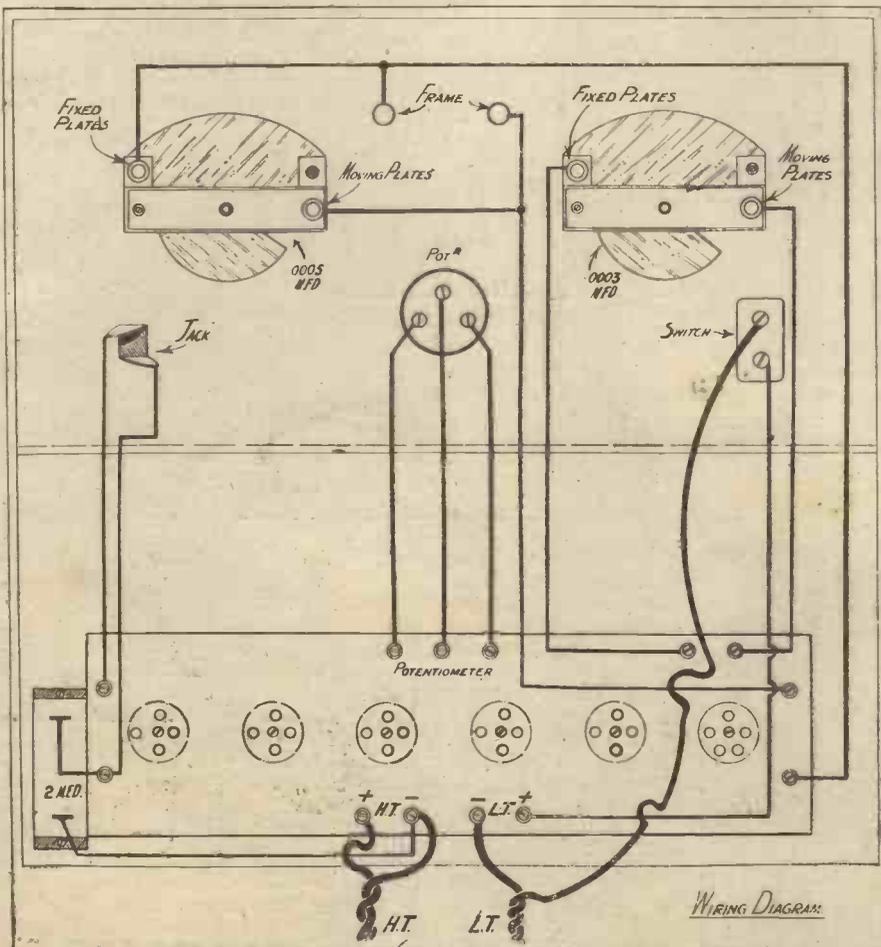
Wiring is of the simplest character. Note that the conventional terminal strip is unnecessary.
