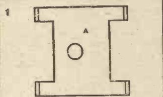
The heavy Gauge main frame "A," shaped to eliminate self-capacity and placed well out of magnetic field, avoiding eddy current losses.
