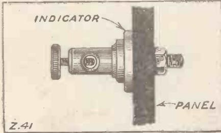
green on the negative. Next you will have to screw the terminals to the panel by means of the nuts, as shown in the sketch. These counters are likely to be made of bone, and thus prove to be excellent insulators for a wood panel if one is placed at each side of the panel.
