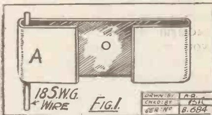
of the strip, it is a good plan to press the pieces together (using pliers) over a bit of 18 S.W.G. wire inserted at the points marked A. This gives a certain springiness to the clip when the wire is removed.
