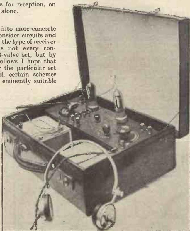
A two-valve portable set constructed by the author.
