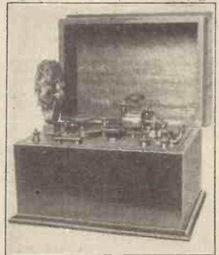
An elaborate form of crystal receiver providing for the use of many different circuits.
