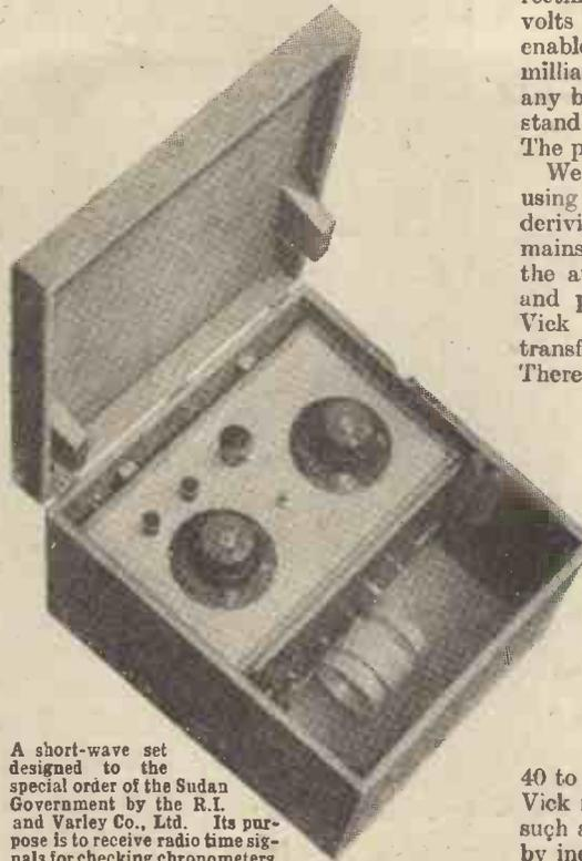
A short-wave set designed to the special order of the Sudan Government by the R.I. and Varley Co., Ltd. Its purpose is to receive radio time signals for checking chronometers.
