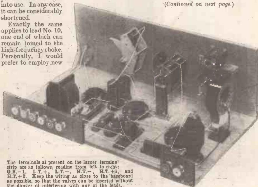
The terminals at present on the larger terminal strip are as follows, reading from left to right: G.B.-1, L.T.+, L.T.-, H.T.-, H.T.+1, and H.T.+2. Keep the wiring as close to the baseboard as possible, so that the valves can be inserted without the danger of interfering with any of the leads.
