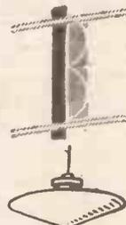
Another way of utilising the cone diaphragm method of construction.
