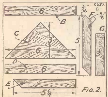
to attach to each the pieces of wood shown in Fig. 2, which gives the necessary dimen-
