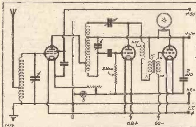
Here is the modernised "Melody Maker's" circuit—screened-grid high-frequency amplifier, detector, and transformer-coupled L.F. stage.
