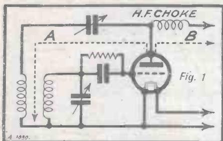
their way down to filament, and you will see that in the circuit sketched there are two paths which they can take, marked A and B. A is the normal reaction path through the reaction condenser and the reaction winding, while B is through the H.F. choke, through the phones, intervalve transformer primary or what not, and so to the H.T. battery and down to filament.
