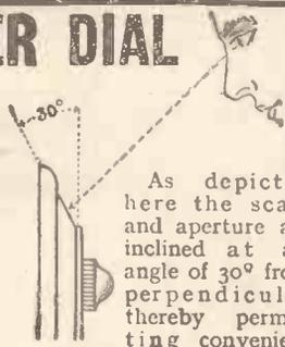
As depicted here the scale and aperture are inclined at an angle of 30° from perpendicular thereby permitting convenient unobstructed view of scale without need to crouch or stoop.
