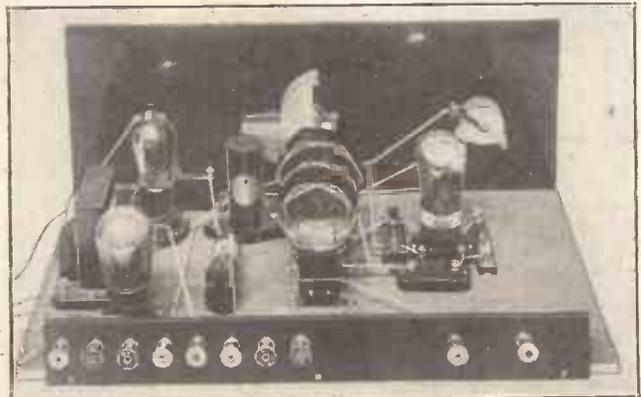
Three plug-in coils are used for tuning and reaction, the L.F. side being resistance-transformer coupled.
