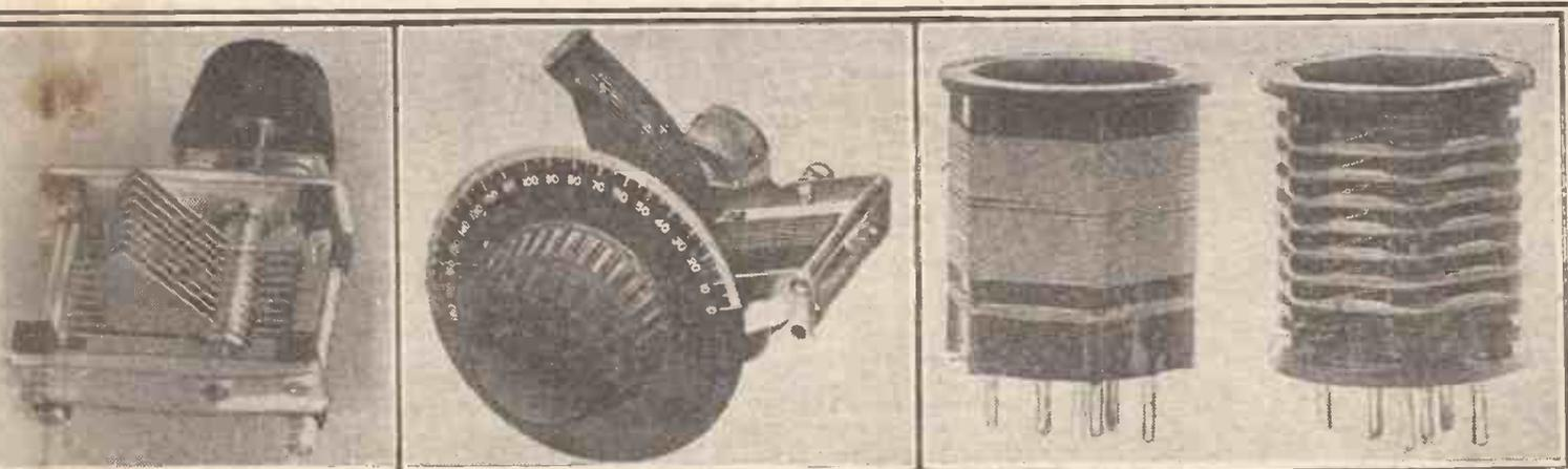
Special Formo 6-pin dual range coil unit. The tuning components on the right hand page are, left to right, the Bowyer-Lowe reaction condenser, an Ormond slow-motion tuning condenser, and a slot-wound long-wave coil.
