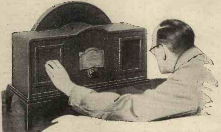
The picture appears at the back of the aperture at the right, and it is difficult for more than one or two people clearly to view it. The synchronisation is adjustable by a knob on the left, and this knob requires very careful adjustment indeed. The centre knob is for "framing" the pictures.
