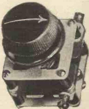
An insulating spindle is a feature of this Burne-Jones component.
