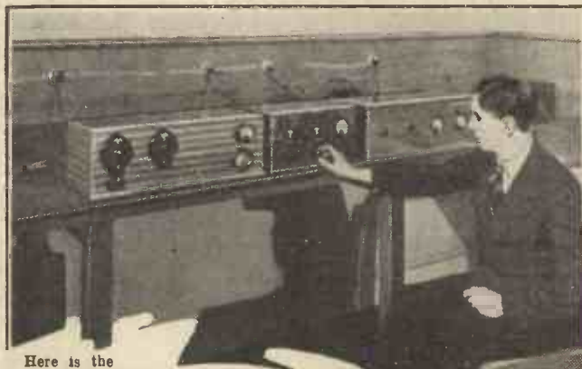
Here is the elaborate laboratory model of the Radiostat. It is capable of tuning-in stations that are being heterodyned, without any interference being heard.
