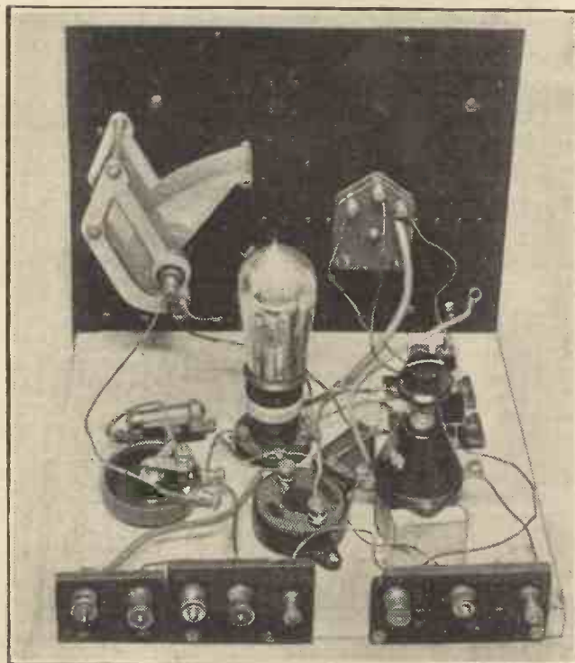
The short-circuited grid condenser can be seen clearly in this plate. Note the very untidy wiring and how the layout of components has been seriously varied from the specification.
