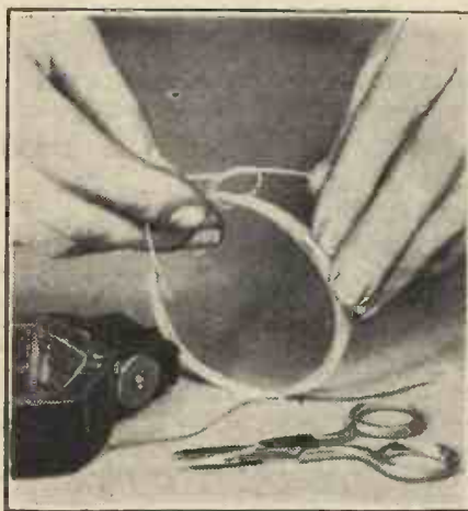
One of the best ways of sharpening tuning is to use a separate aerial coil. If your set hasn't one, you can easily roll 20 turns or so of coil wire into a hank, as shown, tying it with string (not wire) to form an aerial coil. The method of using is shown in "Captain Eckersley's Query Corner" on another page.
