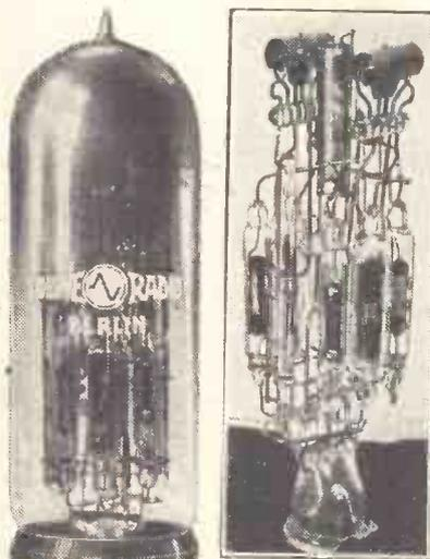
The Loewe 3NF (det. and 2 L.F.) valve, and the interior of the same valve showing the arrangement of electrodes, resistances, and capacities.
