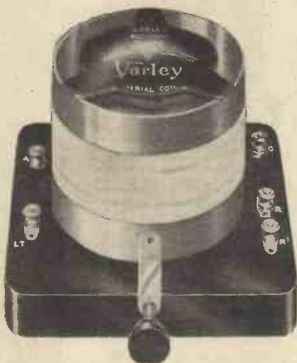
The Varley wave-change coil has an ingenious switching arrangement which enables the controls of a series of coils to be ganged and operated from a single knob.
