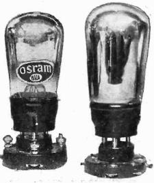
On the left we have the newest Osram valve—the H2, a 2-volt valve baying an impedance of about 35,000 ohms. On the light is the famous Mazda P.220A.
