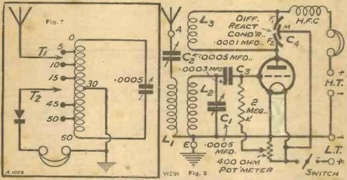
A crystal set based on Fig. 1 gives unusually good long-distance results because the crystal and the aerial connections are tapped (by means of erocodile clips) on to the main coil. This consists of 60 turns of 24 or 26 D.C.C. wire wound on a 3-inch tube, and tapped at the turn numbers shown.
