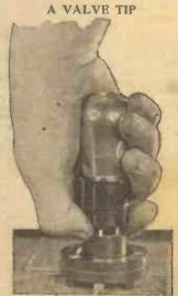
Don't pull on the glass or you may loosen it. Get a grip on the base as well before pulling out a valve.
