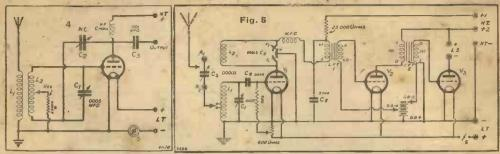
The H.F. Unit (Fig. 4) employs plug-in coils, L, being a 25 or 35, or for long waves a 75 or 100. L, is a centre-tapped coil, 60 for ordinary and 250 for long waves.
