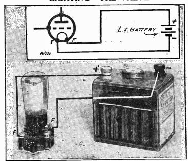
The filament (an L.T.) circuit of a valve. There is a slight discrepancy between the theoretical and pictorial representations. Can you spot it?
