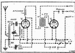
Here are the connections for the simple two-valver, e "parts" for which were given in last week's the "parts"
