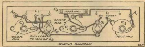
The wiring is very easy, but should be carried out with care in accordance with the above plan.
