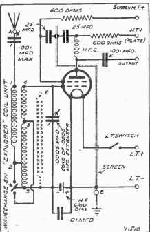
This is the completed diagram, showing that the two "missing" components last week were the grid-bias battery and its by-pass condenser.
