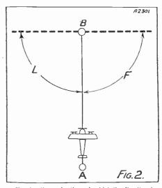
Showing the angles through which the directional station transmits in relation to the correct course.
