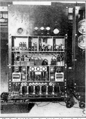
After the reflected light from the subject has fallen on the photo-electric cells the above amplifier magnifies the electrical impulses and passes them on to the transmitter.
