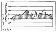
Although the voltage-amplification variations shown look very nasty, it is unlikely that even a keen ear would hear the difference between these and a completely straight-line response.
