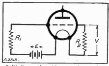
In this diagram the resistances are shown as they appear in a circuit in practice. R<sub>2</sub> represents the valve's impedance between grid and filament, and R<sub>1</sub> the value of the grid leak through which the bias is applied.
