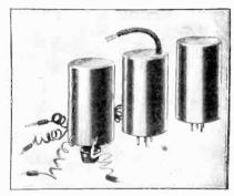
The LEWCOS Super-Het Coil Kit (Reference S.H.K. No. 3) (protected by provisional Patent Specification).
