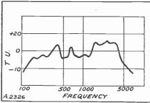
The response curve of an ordinary cone loud speaker plotted against Transmission Units (Decibels), a system which gives a closer approximation of what is heard than straightforward degrees of overall voltage-amplification.
