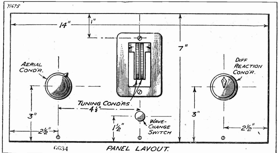
There are only four panel components to mount, and easy dimensions make the marking out of the positions for the holes a simple matter. Note that there is no on-off switch, all the "on-offing" being done from the unit.
