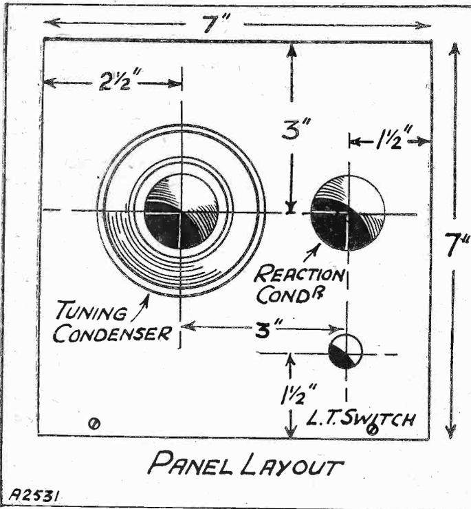
The panel is quite a small affair, and there are only three controls. Most panel components are arranged nowadays for one-hole fixing, so it should only be necessary to drill the ebonite at the places marked. All the measurements are clearly indicated.
