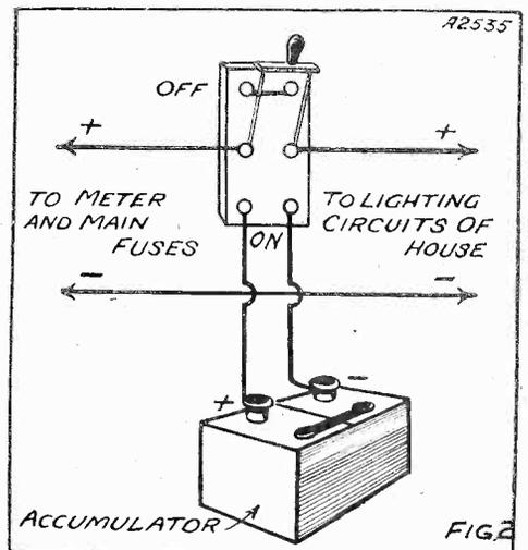
"Free" L.T. accumulator charging can be obtained by connecting the battery in the house-lighting circuit. There is no noticeable diminution of light from the lamps.
