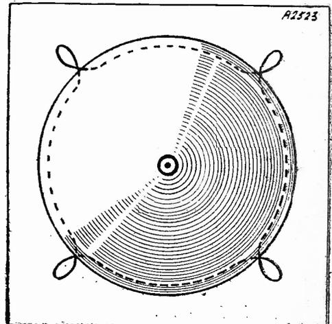
The cone is supported by the four loops, the string being continued round the periphery and glued firmly in place.
