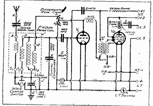
This is the simple circuit given last week, with the three "missing" components inserted. It will be seen that these were all condensers—a 2-mfd. for decoupling, a '0003-mfd. grid condenser, and a 2-mfd. for the output circuit.
