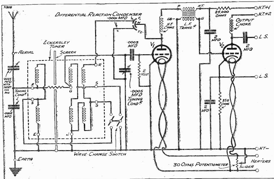
The simple nature of this all-from-the-mains receiver is largely due to the use of a separate unit for the power supply instead of incorporating all the "mains" components in the receiver proper.
