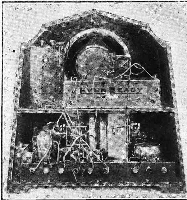
Now that the practice of concentrating batteries, set and loudspeaker in one cabinet has become so common it is worth bearing in mind that if box resonance is to be avoided, it is a good idea to leave the set open behind. Or if you have a back, see that a number of large holes are drilled in it.
