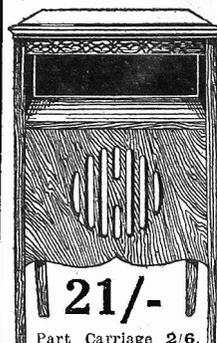
polished a rich nut-brown shade, this Cabinet stands 35 inches high. The panel space measures 18 x 7 ins., while the top is 21 ins. wide by 14 1/2 ins. deep. The loudspeaker aperture is 10 ins. diameter and is covered with fine amber silk. There is a removable panel back giving free access to batteries and speaker. The deep-hinged lid enables the set to be removed bodily. Decide now to have this fine Cabinet in your home. Money back if not entirely satisfied.
