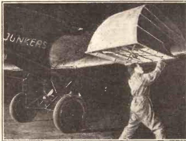
Making adjustments prior to a night test of "the flying loudspeaker." Fixed to the wing of an aeroplane this speaker can be heard over nearly a square mile, when the machine is flying at about 1,000 feet, and tests of its advertising value are being carried out in Germany.
