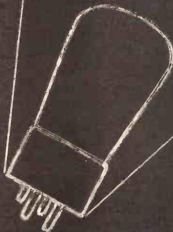
So simple and yet so efficient. One discovery, the Mullard "non-vibrating filament," has made the greatest advance in modern valve construction — microphony has been overcome.
