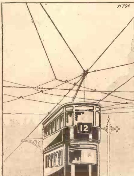
The overhead trolleys of cars produce a lot of electrical disturbances.
