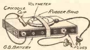
Continuity tests can be carried out quickly with this "gadget."
