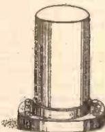
The can on a screened coil should be earthed.
