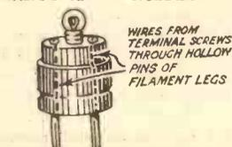
Don't risk your valves in a new receiver when this simple filament tester is so easy to make.
