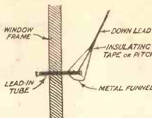
The insulating tape at the top of the funnel keeps out the rain.
