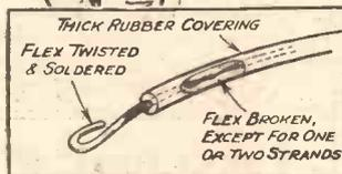
Careful search is needed to find a fault in a flex lead because of the rubber casing.
