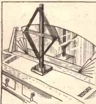
For a frame having sides one yard in length, six or seven turns will be needed to cover the usual broadcasting wave-band between 200 and 600 metres. Bare or covered wire may be used, and 22 D.C.C. wire, as recommended for indoor aerials, will do admirably
