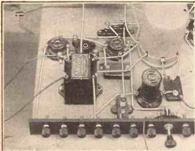
This photograph of part of the baseboard, and the sketch to the right, show how the pick-up switch and wiring are arranged. In the sketch, the dotted line represents the original connection, and the black lines indicate the new leads.
