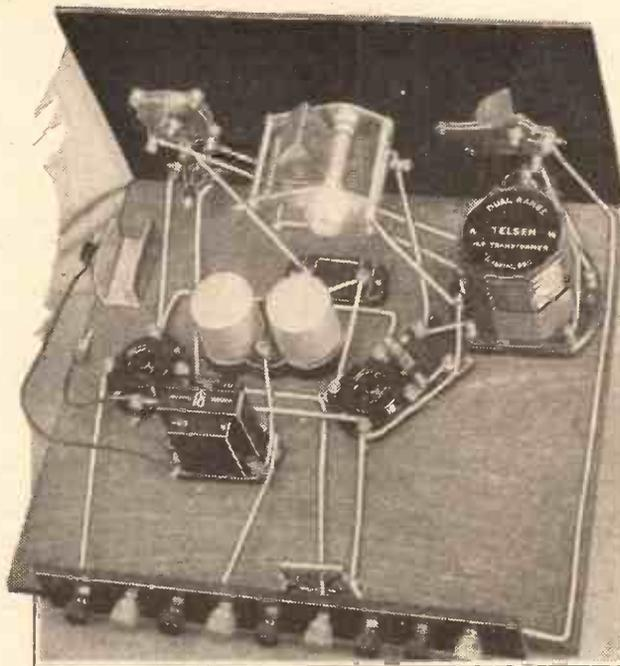
There are no sub-baseboard parts or wires—every component and wire is "above board."
