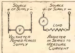
Voltmeter and ammeter readings are taken with quite different connections for the meters.
