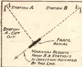
The frame should be exactly in line with the station for best results.
