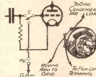
The grid circuit type radiogram change-over switch with its theoretical connections.
