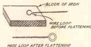
A flat loop in wiring leads will not open out.
