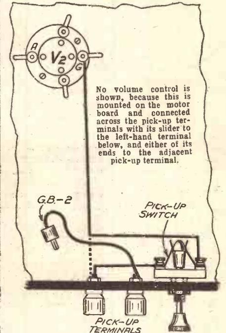
No volume control is shown, because this is mounted on the motor board and connected across the pick-up terminals with its slider to the left-hand terminal below, and either of its ends to the adjacent pick-up terminal.
