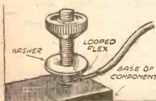
A washer on top of a looped flex end will simplify tightening.
