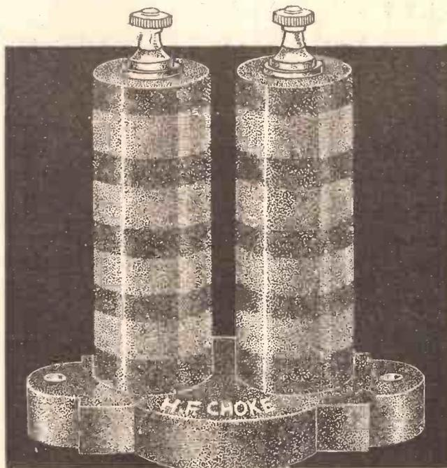
Igranich Binocular type of H.F. choke . . . a good choke and suffers from no peaks over its rated range of 150 to 2,500 metres . . . in view of its indisputable technical attractions, it is good value for money.
