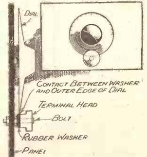
See that the rubber washer and not the terminal head makes contact with the dial.
