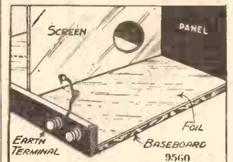
Joining screens by a special lead ensures their proper bonding.
