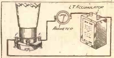
The resistance of an ammeter is very low, and so does not upset the current flowing in a circuit.
