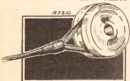
A tapering effect is obtained by employing the fastening-off method illustrated here.
