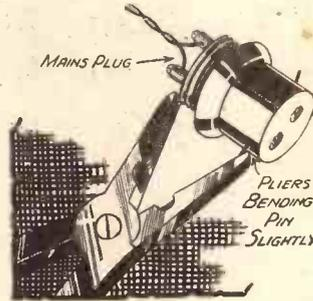
on the plug not being firmly held against the spring-loaded plugs in the holder. This is often due to the bayonets being too near the end of the plug.
