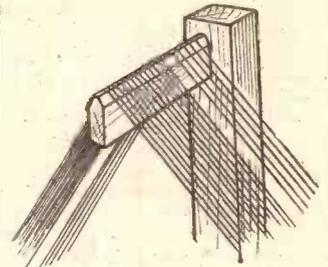
Slots cut in the corner piece provide simple spacing of wires.
