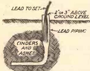
Note how the pipe is flattened over the insulation to keep water from rotting the wire.
