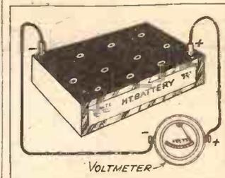
The positive terminal of a voltmeter should be connected to the positive terminal of the battery.
