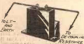
One side of the condensers used with decoupling resistances usually goes to earth.
