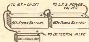
The power of the two super batteries is kept even.
