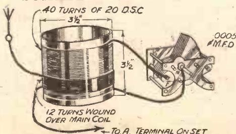
Many constructors will have the necessary parts and materials on hand for making this wavetrapping.
