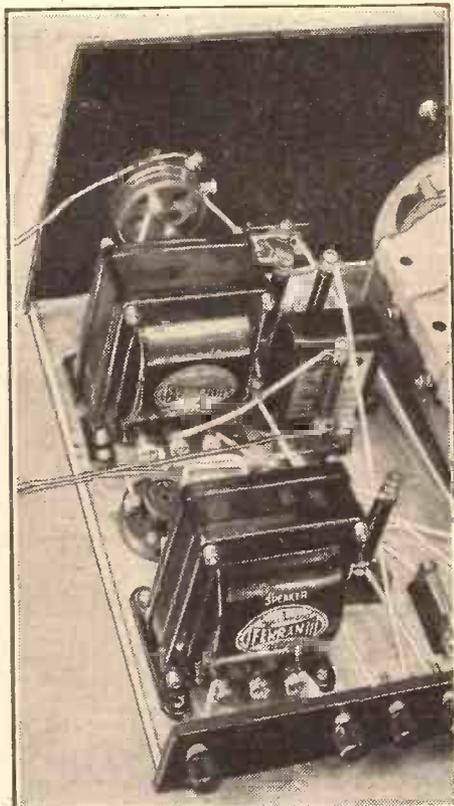
The L.F. end of the "Ferro-Q," showing the Q.P.P. input and output transformers. The output transformer has a tone compensating resistance and condenser across its primary winding. The variable-mu potentiometer can be seen on the panel.
