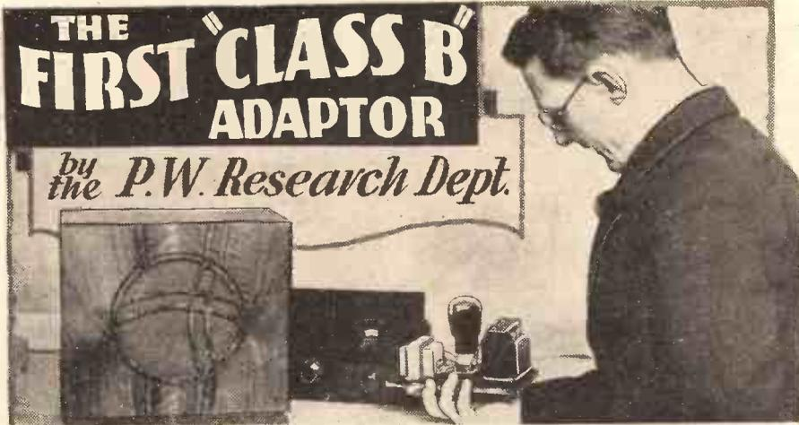
**M**ORE power; less average H. T. current consumption! That is what "Class B" amplification offers the battery-set owner. And here is a compact, easy-to-build adaptor that will enable any listener who has a one-L.F.-stage battery set to try "Class B" without any but the most trifling alterations to his set connections.
