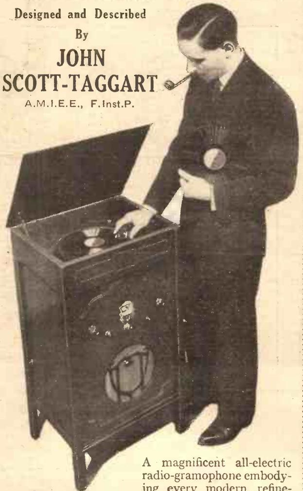
A magnificent all-electric radio-gramophone embodying every modern refinement including iron-core coils, ganged tuning and pre-detector volume control.
