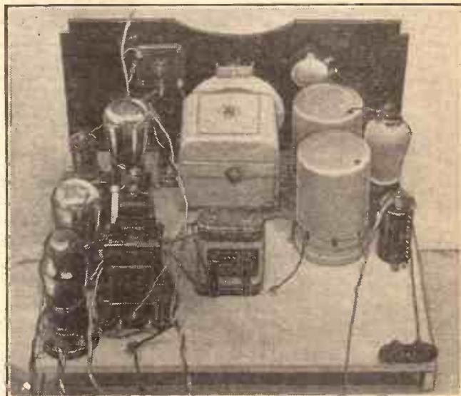
That the construction will present no difficulties to even an inexperienced builder will be immediately apparent from this rear view of the completely wired panel and baseboard assembly.
