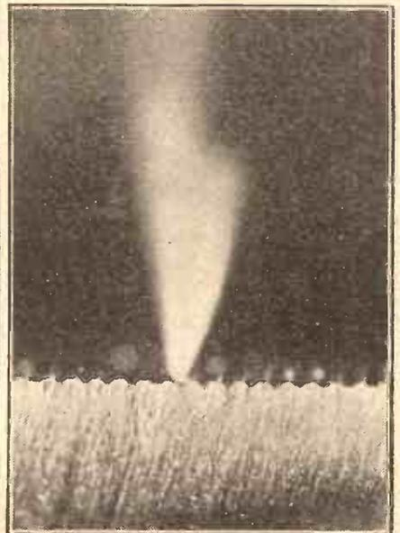
This greatly enlarged photograph depicts a steel needle resting in one of the grooves of a record. A worn or faulty point will cause damage to the grooves and considerably shorten the life of the record.
