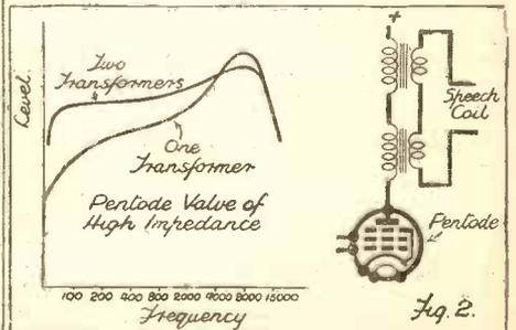
Showing how you can get more bass by using a higher anode impedance in the form of two transformers in series, as shown, provided the valve has a high impedance.
