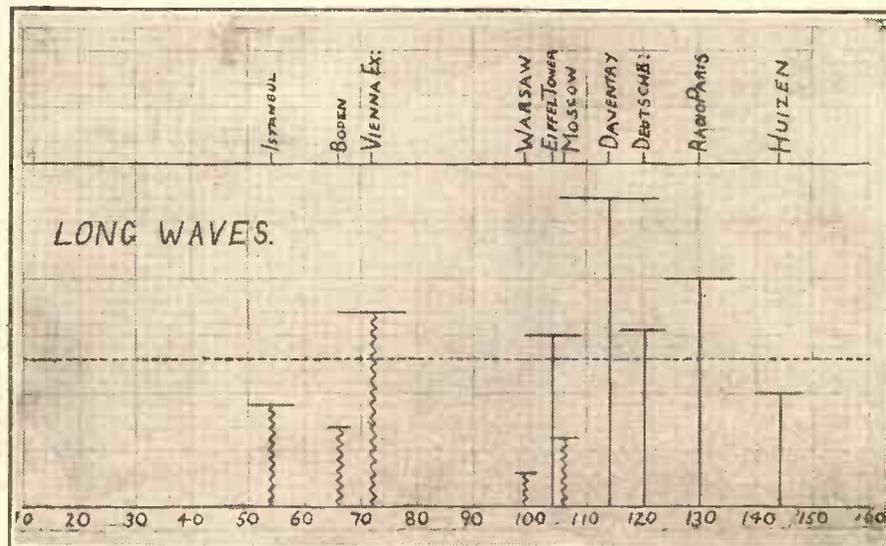
This chart was drawn up to represent daylight reception on the long waves. The dotted line indicates the division between stations that need reaction and those which do not.
