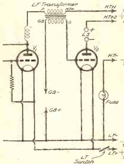
A portion of the circuit of a recent “P.W.” receiver (the “Unity” Two) is here used to illustrate our Radio Consultant’s explanation. The H.T. electrons start at the negative point -1 and flow through the filaments of the valves V1 and V2, returning to the positive terminal of the H.T. battery through the points marked +3 and +4. Similarly, the L.T. electrons flow from point -2 through the filaments of the valves V1 and V2, back to the positive L.T. point marked +2.
