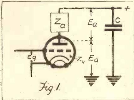
If to any valve you apply  $E_g$ , a voltage to the grid, and this voltage is magnified by the valve acting with  $Z_a$  (the anode impedance), to give  $E_a$ ,  $E_a$  divided by  $E_g$  is the practical magnification of the valve and circuit combined.
