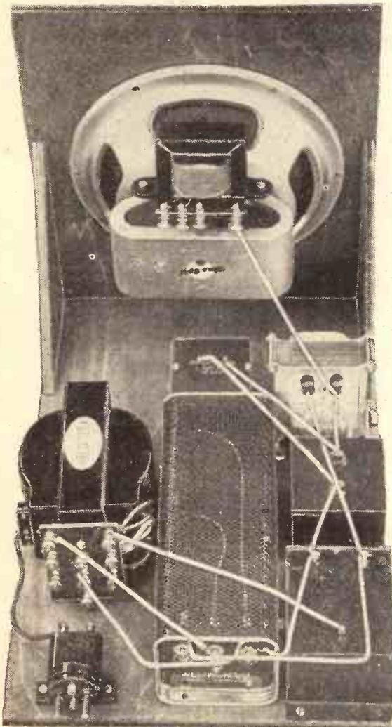
The Power Pack for the "Double X" also contains the loudspeaker and fits in the cabinet beside the chassis. It is best to connect up the two sections before they are pushed right into the cabinet.
