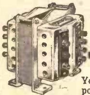
You need only three components, a Heayberd Mains Transformer, Westinghouse Rectifier, and a small Resistance, all of which can be obtained from Heayberd. The cost is as low as 32/-. This charger will last you years, and will be an interesting introduction to radio assembly.
