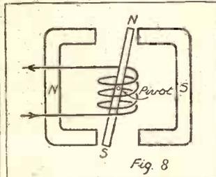
If the direction of the current through the coil is reversed, the upper end of the armature becomes a N. pole. Like poles repel, so the armature swings over to the right.
