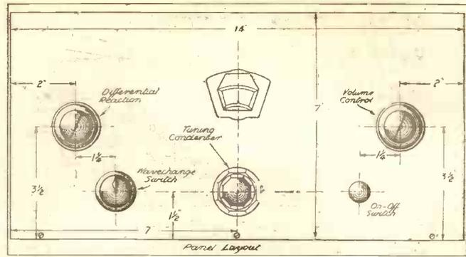
Tuning is a particularly easy operation, since the aerial circuit tuning adjuster is brought out to a small knob concentric with the main tuning control.
