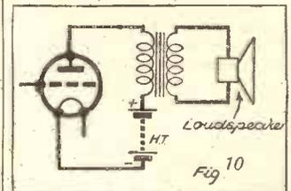
With a true balanced-armature loudspeaker it is desirable to use an output filter, such as a transformer, and so isolate the speaker from the anode current.
