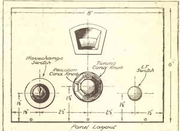
Apart from the two switches, there is only the centre control, the larger knob of which adjusts the tuning, while the smaller one "looks after" reaction.
