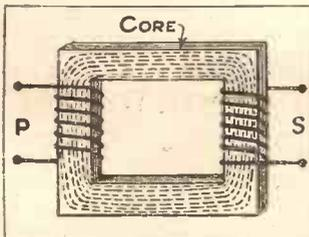
Fig. 1. A transformer in its simplest form. Two coils of wire, P and S, are wound round the core as shown.
