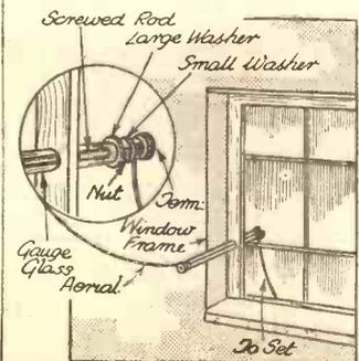
The glass lead-in tube shown in this diagram is quite easy to make.
