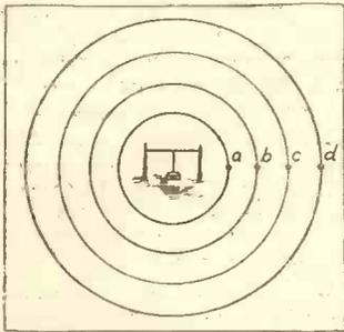
Fig. 1. The waves radiated from a broadcasting station get weaker as their distance from the transmitting aerial increases. Thus the strength of the waves at "a" is greater than at "b" and much greater than at "c" and "d."
