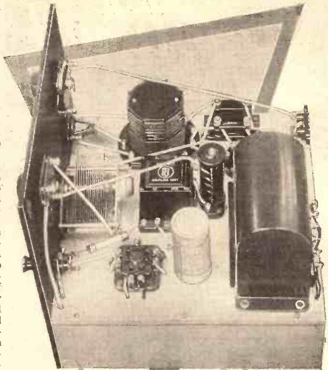
The output valve has a seven-pin base and needs one of the new seven-socket valve holders. The output choke, on the right, is of the tapped variety, and should be "adjusted" to suit the loudspeaker.
