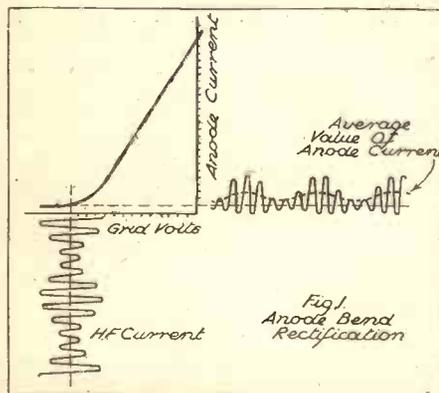
This is the grid-volts/anode-current curve of a valve suitable for anode-bend rectification. For best results the grid bias should be adjusted so that the operating point falls on the bottom part of the curve.
