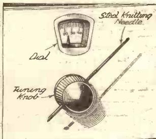
When drilling the knob do not touch the grub screw.
