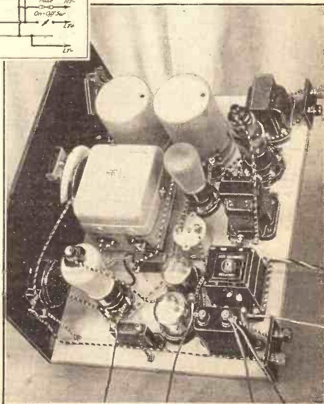
The S.G. valve is the one in the foreground. The valve near the coils with the anode cap being the new driver-B amplifier.
