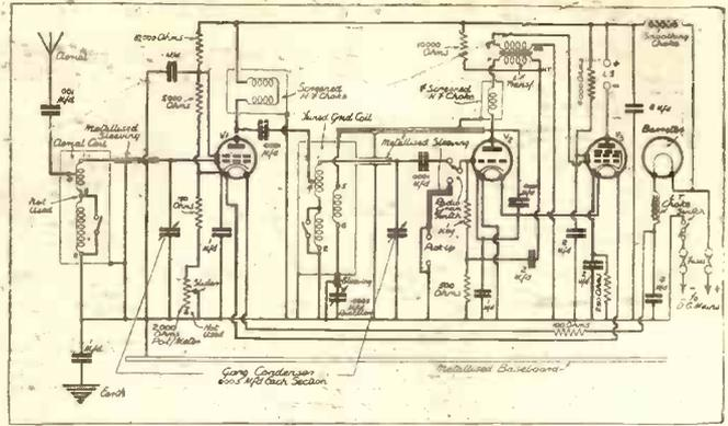
The specially marked leads in this diagram show clearly the main connections which have to be shielded.
