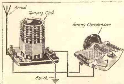
In this pictorial diagram of a simple tuning circuit the connections between condenser and coil, in relation to the aerial and earth, are made clear.
