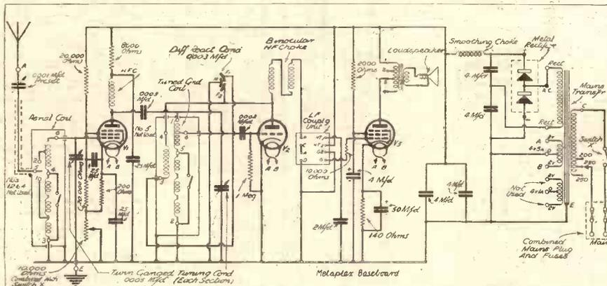
The circuit responsible for the astounding results of the A.C. "Double X." It has a screen-pentode H.F. valve and a specially sensitive output pentode. The two 4-mfd. condensers in parallel between the smoothing choke and H.T. were chosen instead of an 8-mfd. in order to ensure easy availability.
