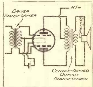
This theoretical circuit of the output stage of a receiver using Class B shows the centre-tapped driver and Class B output transformers and the Class B valve with its two anodes and two grids.
