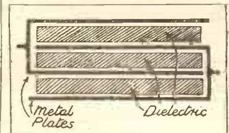
This practical illustration shows how the metal plates are separated by a dielectric, usually mica, paper or ebonite, in a fixed condenser.
