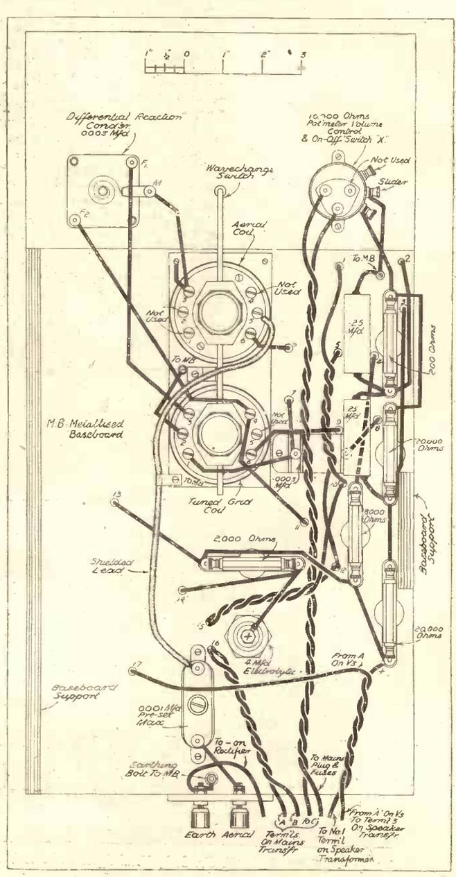
The left-hand diagram shows the above- and the right-hand and the below-base-board layout and wiring of this remarkable three-valver. Some leads go through the wooden chassis, and the holes are numbered so that it is an easy task to correlate the two diagrams.
