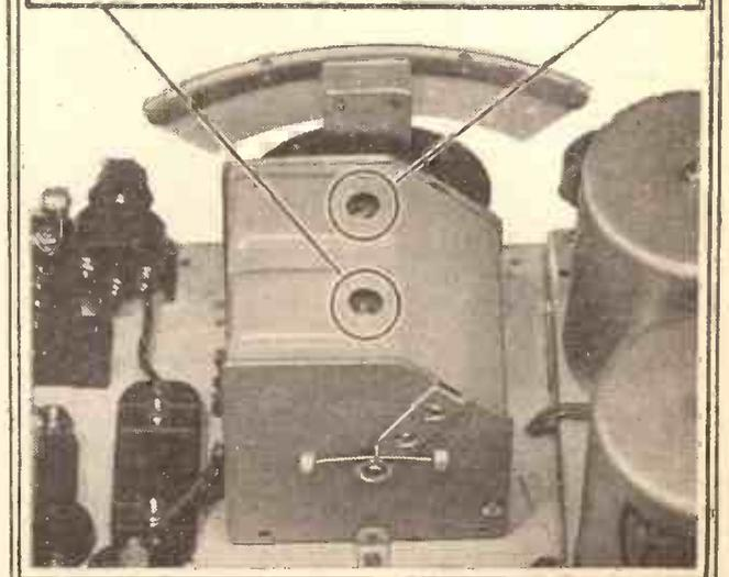
The moving vanes of the two-gang condenser are automatically earthed to the metallised chassis.
