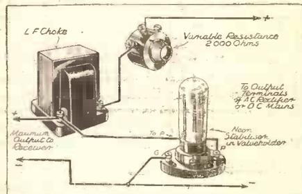
When H.T. is derived from the mains for a Class B receiver, it is advisable to use a voltage stabiliser across the mains unit as shown.
