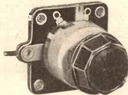
A potentiometer (available in several values) is ganged to a '0003-mfd. reaction condenser in the new volume control in the Utility range of components.
