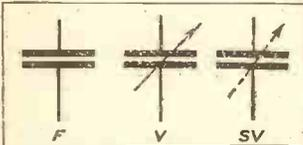
Symbols used to show various forms of condenser in a theoretical circuit. F is a simple fixed condenser. V shows a variable type such as is used for tuning. SV is a semi-variable condenser, also known as a preset.
