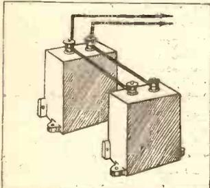
Connecting two condensers in parallel gives a total capacity value equal to the sum of the two individual capacities.
