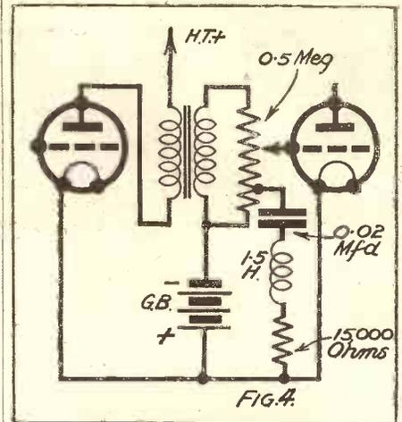
The compensated volume-control arrangement described by the author is not only applicable to resistance-capacity coupling. Where an L.F. transformer is employed the arrangement shown above is recommended.
