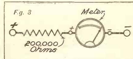
In this third example H.T. voltages up to 200 volts can be read on the same meter by the use of a 200,000-ohm resistance in series.
