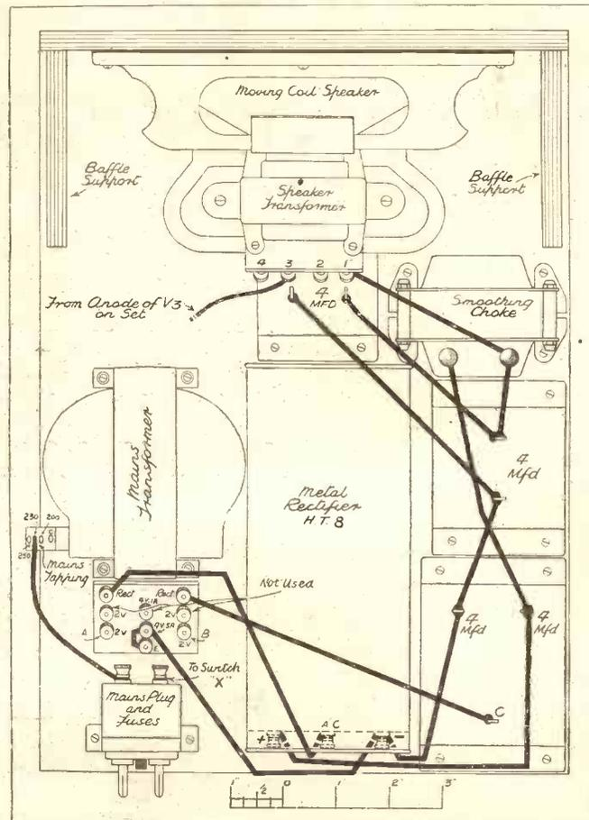
In connecting the power pack to the set, one lead from the on-off switch on the latter is joined to the terminal marked "X" on the diagram—i.e. to the one side of the mains plug. The other switch lead is taken to "G" on the mains transformer input side. The photograph shows only the leads on the power pack itself, and none of the inter-connections between it and the receiver.
