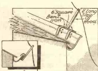
A simple attachment which successfully keeps the aerial lead-in away from the roof.
