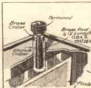
The method illustrated here keeps the terminal well away from acid spray.
