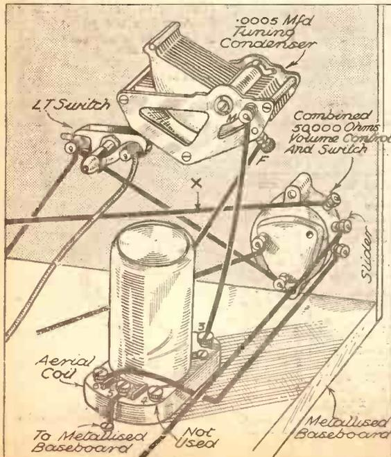
be used for long periods in this condition and provides a highly economical form of reception, too. If more volume is needed and a tour round the foreigners desired, a touch of the volume control brings in the S.G. H.F. valve and the sensitivity of this is adjusted in exact accordance with the requirements—all this with the one little knob.
