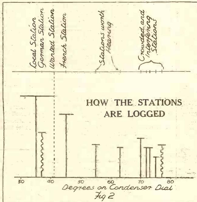
The dotted line represents the position of a wanted station. As it is right on the edge of the local station's spread, obviously it is not likely to be received very well.
