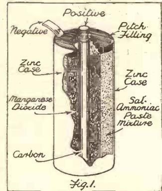
*Fig. 1. The construction of an H.T. battery cell is clearly shown in this sectional drawing.*
