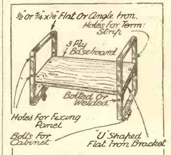
A set built on this type of chassis is particularly accessible.
