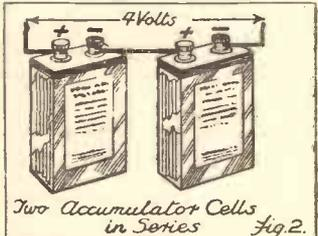
*Fig. 2. Two Accumulator Cells in Series.*
