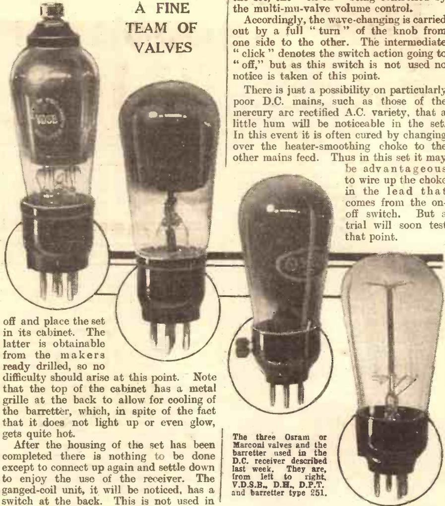
The three Osram or Marconi valves and the barretter used in the D.C. receiver described last week. They are, from left to right, V.D.S.B., D.H., D.P.T. and barretter type 251.
