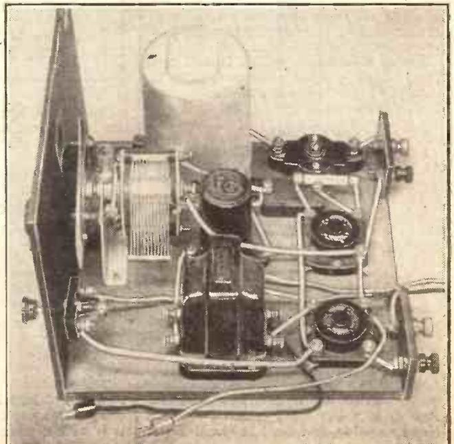
The main feature of the construction is its sheer straightforwardness. The two wander-plugs in the foreground plug into the grid-bias battery, which is accommodated on the side of the cabinet.
