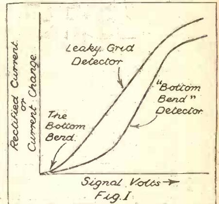
The bottom bend of a typical valve characteristic is shown in the diagram above. The curve on the left represents leaky-grid detection, while the other shows anode-bend rectification.
