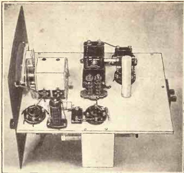
A side view of the receiver showing the general layout of the upper side of the baseboard, and the wooden support that is used on the inner side (nearer power pack) of the chassis.
