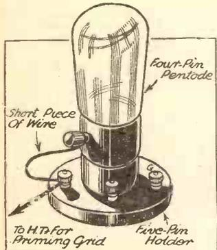
The flex lead  $\frac{1}{2}$  enables side-terminal pentodes to be used in addition to the 5-pin variety.
