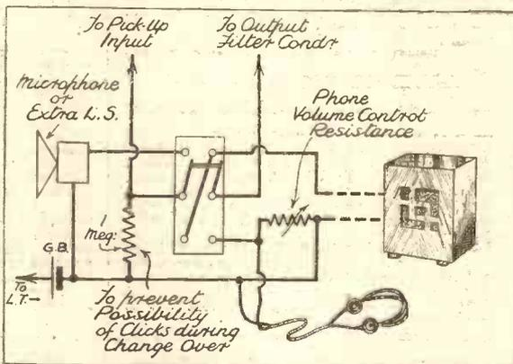
These are the connections you have to make. They are all external to the receiver itself, which can still be used for radio simply by altering the position of its radiogram switch.
