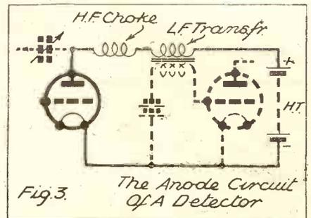
The anode circuit of a valve includes everything which is in the path of the H.T. current on its way from the anode through the H.T. battery to the cathode.
