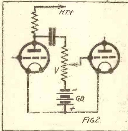
A favourite method of controlling volume on the L.F. side of a receiver is to employ a potentiometer as the grid resistance in an R.C. coupled stage.
