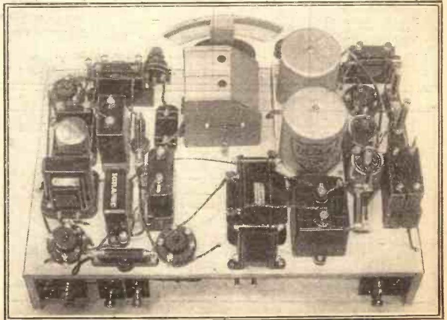
The large choke in the centre foreground is for smoothing the heater supply, and is essential to hum-free operation of the set.
