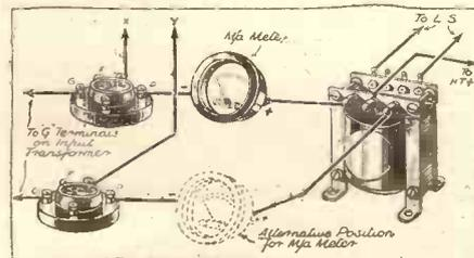
The Q.P.P. valves should be "matched" by means of the anode current test. "X" and "Y" are the two priming grid leads and are joined to H.T. +.
