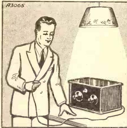
The total H.T. taken by your set can be ascertained with a milliammeter joined in the H.T. negative lead.
