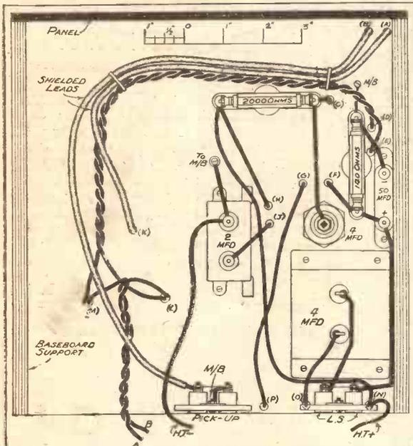
The screened leads and the twisted flex heater connections run mainly below the wooden baseboard, which is sprayed with metal to form a screened chassis.
