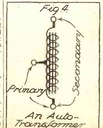
An auto-transformer consists of one winding only, different ratios being obtained by arranging suitable taps.
