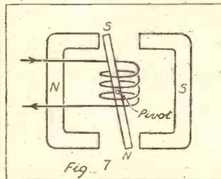
When a current passes through the coil in the direction shown, the top of the armature becomes a S. pole. Therefore, as unlike poles attract, the armature swings over to the left.
