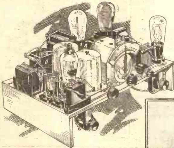
There are only three valves in this D.C. receiver, the fourth "valve" (second from the left) is the vacuum barretter that controls the heater current.
