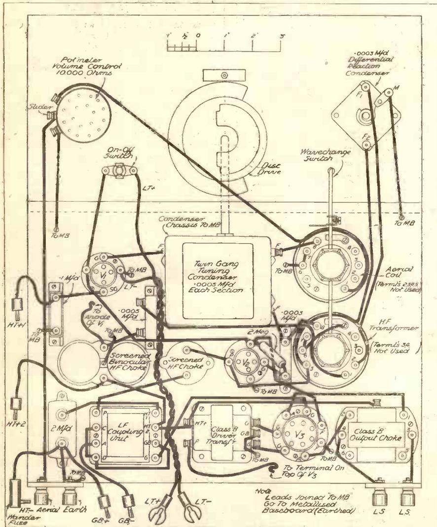
is tuned and connected across grid and filament of the screened-grid valve whose anode is shunt-fed to the primary of the second coil forming H.F. transformer coupling to the detector.
