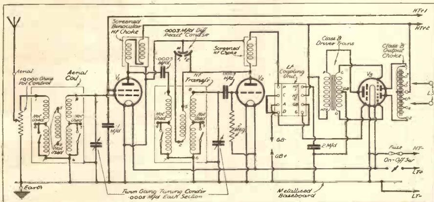
The circuit of the D.B. Three looks perfectly conventional until we come to the L.F. side, when it will be noticed that a new type of output valve is employed. This valve plays the part of both driver and Class B, and is virtually three valves in one envelope.
