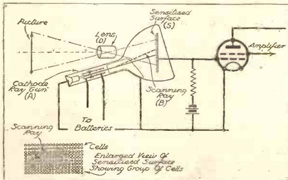
A diagrammatic illustration of the arrangement of the Iconoscope cathode-ray tube and its associated circuit as applied to the transmission of television pictures.
