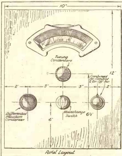
The controls of the receiver present a neat appearance, and require few holes to be drilled.
