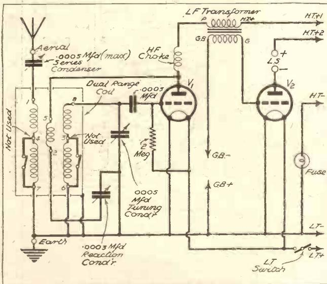
Adjustable selectivity is provided by the pre-set condenser in series with the aerial feed, while the aerial transformer carries the powers of selection of the set still further.
