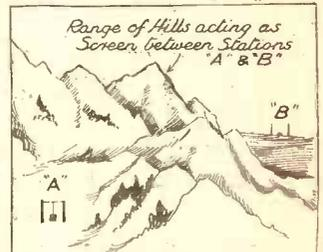
Fig. 3. When there is a range of hills or some other form of shielding between a broadcast transmitter and a receiving aerial the ground wave may get absorbed.
