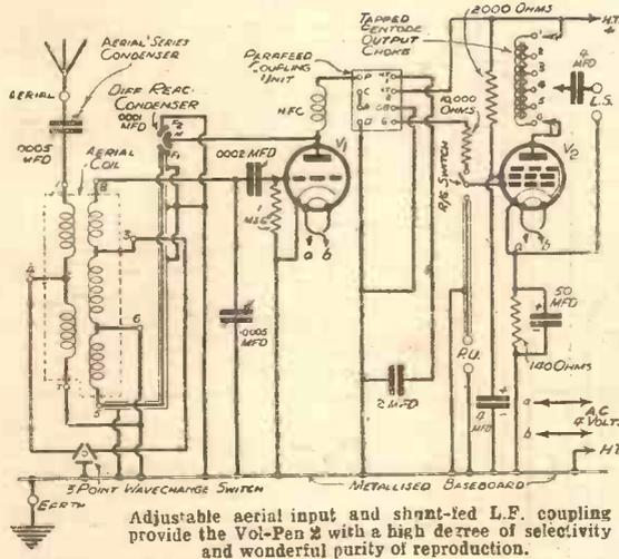
It is well known that in a single circuit, or H.F. transformer-coupled aerial, the selectivity depends on the aerial coupling and the damping of the coils. It may be improved by loosening the aerial coupling and by reducing the damping of the tuned circuit by, say, reaction.
