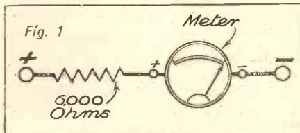
The insertion of a 6,000-ohm resistance, in series with the standard milliammeter, allows readings up to 6 volts to be taken.
