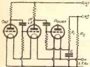
A useful idea for providing automatic grid bias in a battery set.
