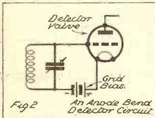
A suitable circuit for anode-bend rectification. A bias of approximately 3 volts is usually required.
