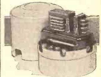
Iron-cored coils are the most recent development in tuning technique. Amongst other advantages, a big saving of space is obtained, as you can see by comparing this photograph with that of an air-cored coil of a similar type.
