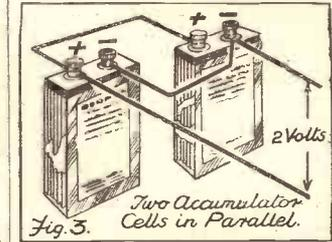
*Fig. 5. Two Accumulator Cells in Parallel.*
