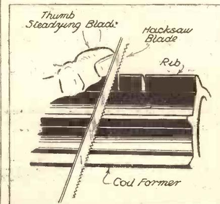
The slots are widened by making a second cut with the hack-saw, at the side of the first one.
