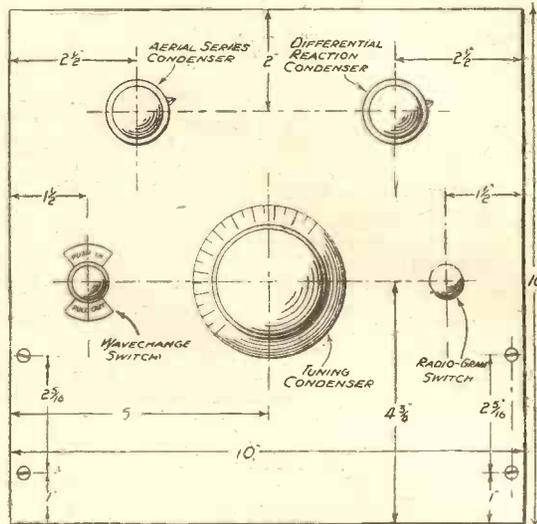
The panel drilling is particularly easy since all the panel components are of the one-hole fixing type.
