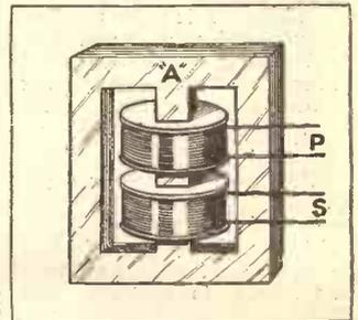
Fig. 2. The core of a commercial transformer is made up of a number of laminations clamped tightly together and insulated from one another.
