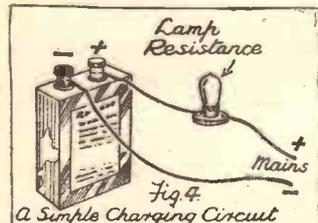
*Fig. 4. A Simple Charging Circuit.*
