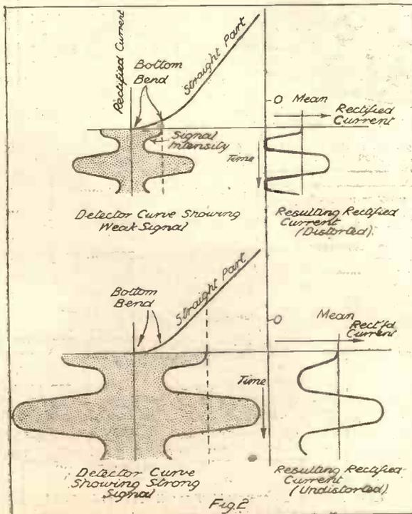
An interesting comparison between the effect of a weak and a strong signal on a detector which has a bottom bend is provided in this diagram. It will be noticed, as pointed out by P. P. E. in the accompanying article, that, while the output from the weak signal is somewhat distorted, that from the strong one remains comparatively unaffected.
