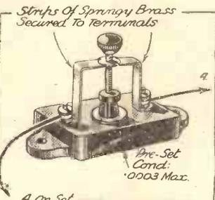
When the condenser is screwed to its maximum position the nut under the knob shorts the two metal strips.
