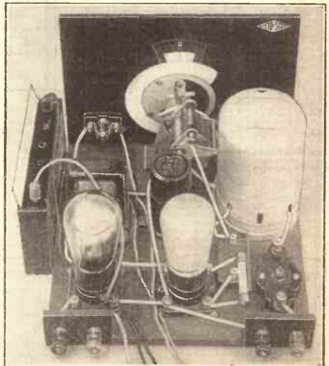
The tuning and reaction controls are carried out by concentric knobs on the main condenser. The screened coil reduces the danger of direct pick-up of a local station by the tuned circuit of the receiver.
