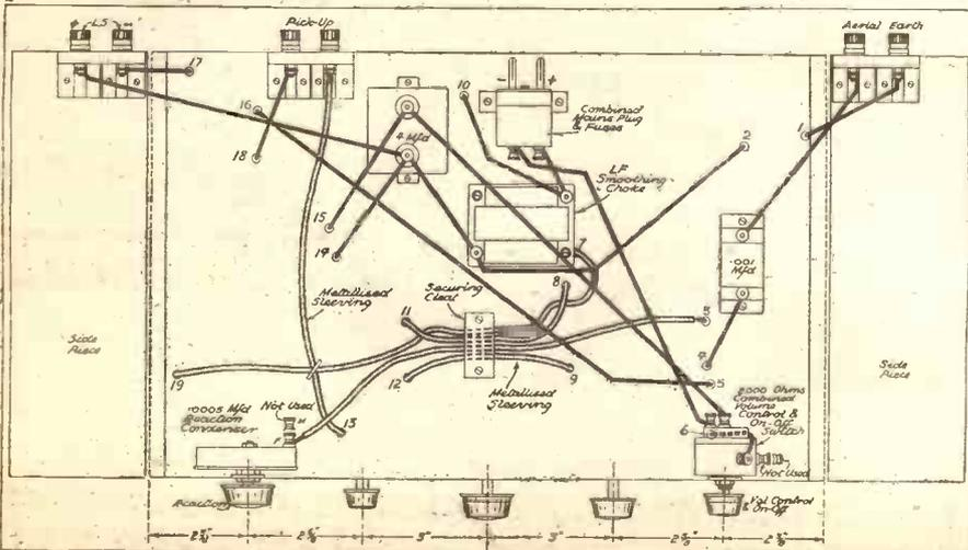
The chassis wiring: when leads go through to the other side of the baseboard the holes are numbered so that the wires can be traced easily.
