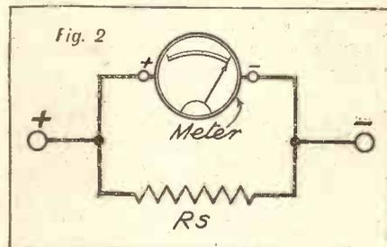
By varying the value of the resistance  $R_s$  the meter can be made to read up to 1 amp. The smaller the resistance the larger the current which can be read by the meter.
