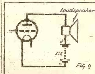
When the loudspeaker is inserted directly in the anode circuit, the steady H.T. current tends to hold the armature to one side. A spring is usually provided to counteract this.
