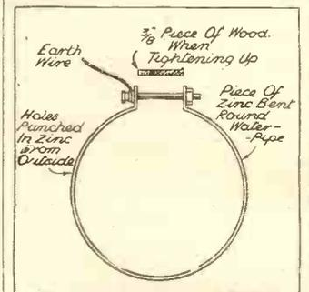
Obtaining a good water-pipe earth will be assisted by this clip.
