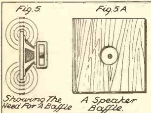
Adding a baffle to a speaker has the effect of improving the low-note response. Without the baffle the sound waves from the front and back of the cone tend to cancel out, meeting over the edge of the chassis.
