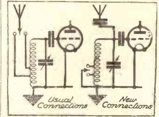
An alternative method of connecting a centre-tapped coil.
