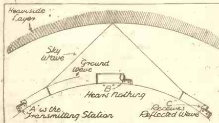
Fig. 2. The sky wave from "A" is reflected by the Heaviside Layer and picked up by "C." But "B" hears nothing because he is not in the path of the reflected wave or within range of the ground wave.
