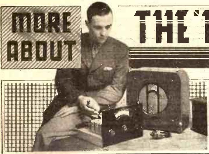
The success of a receiver does not rest merely on its design and its construction by the set builder; the "final touches" play quite a big part in the results that are obtained. In these the matter of trimming the variable condensers is of importance, and the process should be carried out with special care by the constructor.
