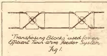
Fig. 1.—Twisted flex is often used for feeders in "noise-reducing" aerial systems. It is preferable, where possible, to use "transposition blocks" of the kind shown in this diagram. One block should be placed at every eighteen inches or two feet, and the feeders may be either of rubber-covered flex or rigid bare wire.
