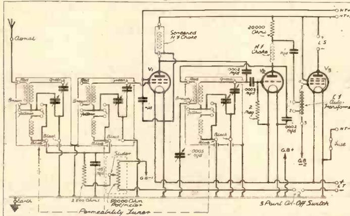
The six "variable condensers" shown across the coils in this diagram are the trimmers and are incorporated in the coil unit. Once set they do not have to be touched. The long-wave and medium-wave inductances are separately trimmed, as was explained last week.
