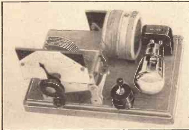
This interesting short-wave receiver, to which W. L. S. refers in the article on this page, was built in 1923. Note the "low-loss" coil, horizontal valve mounting and calibrated dial.
