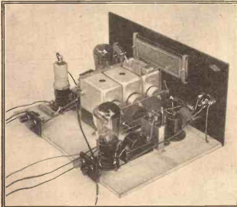
A general view of the "Nu-Tune" Three. Note the iron cores which slide in and out of the coil centres, controlled by the tuning knob on the panel.
