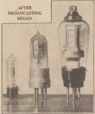
AFTER 1922 we come to such valves as these; The tiny dull-emitter "Wecovalva," the bright-emitter Mullard "Ora" and a Mazda screened pentode of modern design.
