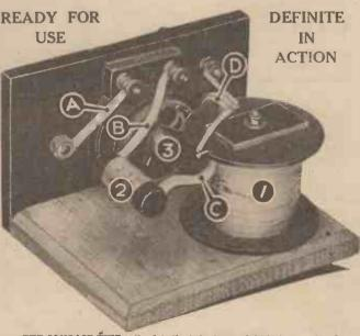
THE COMPACT UNIT. No. 1 is the inductance of 4,560 turns; No. 2 is the '02-mid, condenser; No. 3 is the 10,000-ohm volume control used as a variable resistance. A and B are the leads from the resistance to the pick-up terminal and to the condenser respectively, the former lead going to the slider. C connects the '02-mid, condenser to the end of the coil, and D indicates the three tappings.
