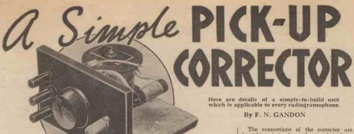
NEARLY every pick-up has what is called a resonant point or "peak" in its characteristic curve, which means that it over-accentuates certain notes in a definite though narrow region of the musical scale. This disproportion is sometimes quite severe, and usually occurs in a part of the scale where it is noticeable to the ear—between 1,500 to 3,500 cycles. A bad peak is usually the cause of that shrill jarring character of certain high notes due to the unbalanced upper register.
