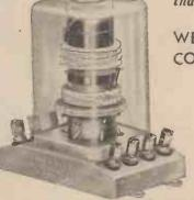
THE WEARITE IRON-CORED WAVE TRAP COIL UNIT
