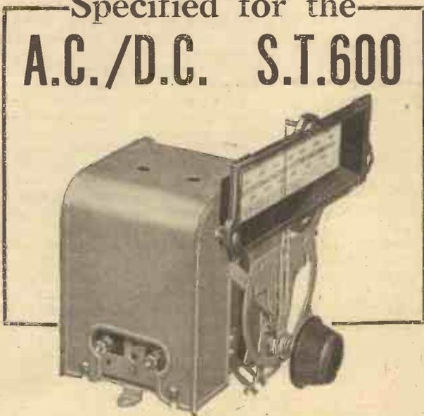
Rigid steel frame with cover, Air di-electric trimmer operated by knob concentrically mounted with tuning knob.
