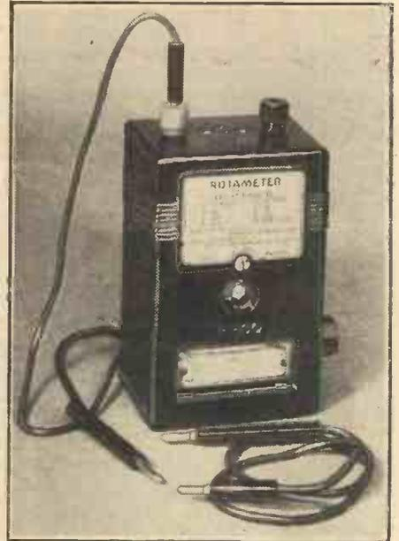
A feature of this Pifco Rotameter-de-Luxe meter is the provision of scales which automatically change with the operation of the range-change switch.
