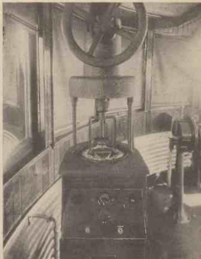
A ship's direction finder. Note the handwheel for moving the loop aerial, which is on the deck above, and the gyroscopic compass for reading the bearings.
