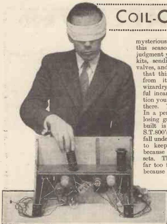
The new self-locating coils used in the S.T.900 are so simple to fit into their holders that this can be done blindfolded with perfect certainty that they can be immediately inserted. Coil-changing takes only a second or two.
