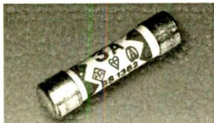
A 1in. 3A ceramic fuse as fitted into most UK mains plugs. They may be sand-filled to prevent internal arcing.
